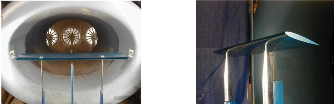
Figure 2 – Photos of the standard airfoil NACA0012 setting in the S4 wind tunnel of ISAE.
