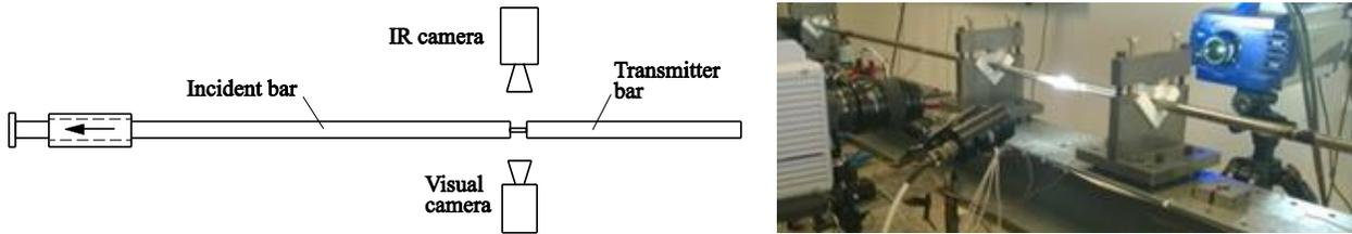
Fig. 7: Tensile Split Hopkinson bar with full-field deformation and temperature measurements.
