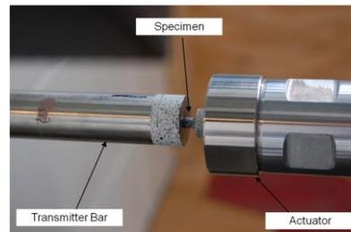
Fig. 3: Intermediate strain rate apparatus.
