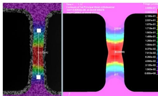
Fig. 5: DIC data and numerical simulation of a tensile test.
