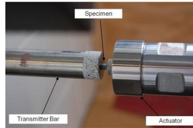
Fig. 3: Intermediate strain rate apparatus.
