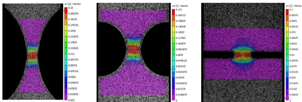
Fig. 6: DIC data from tensile testing of flat-notched-specimens.
