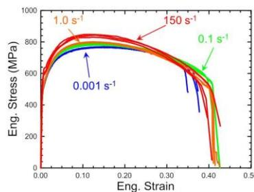
Fig. 4: Tensile stress strain curves for HHS at different strain rates.
