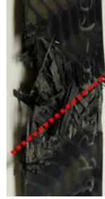
Figure 8. LS-DYNA simulation of 60° off-axis tension simulation; simulation (left) and experiment (right) both show a tensile failure of the bias tows oriented parallel to the applied loading and a failure path in the direction of the axial tows.
