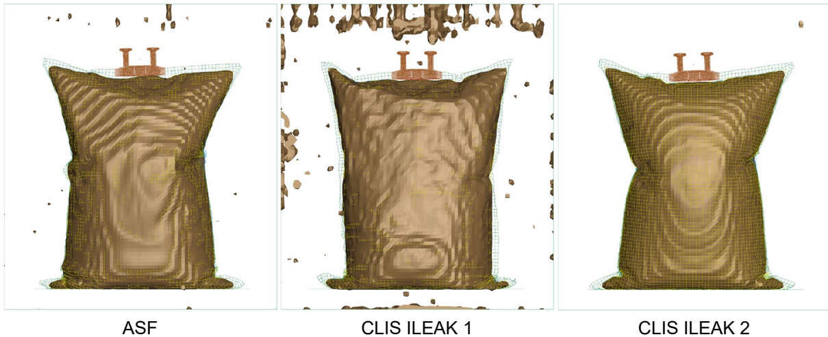
Fig.15: Model state at time 0.215 s: ASF has crushed at that time, CLIS ILEAK 1 shows enormous leakage, CLIS ILEAK 2 works near ideal
