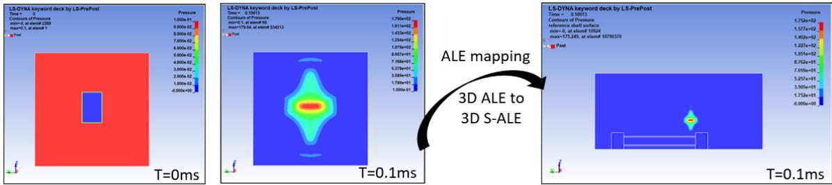
Figure 4: 3D ALE mapping to 3D S-ALE model blast pressure distribution contour
