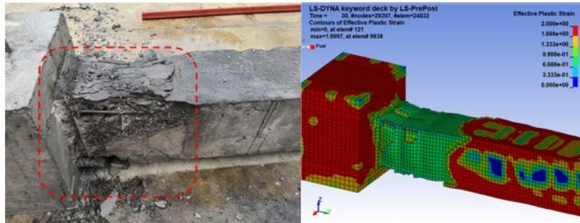
Figure 6: RC beam-column damage comparison against close-in detonation (mesh ratio 4.2)
