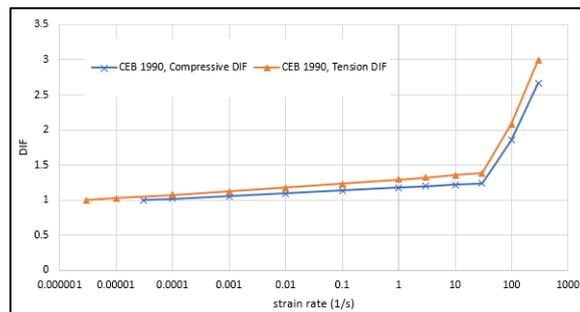
Figure 2: Strain rate effect on the concrete compressive strength of 32MPa
