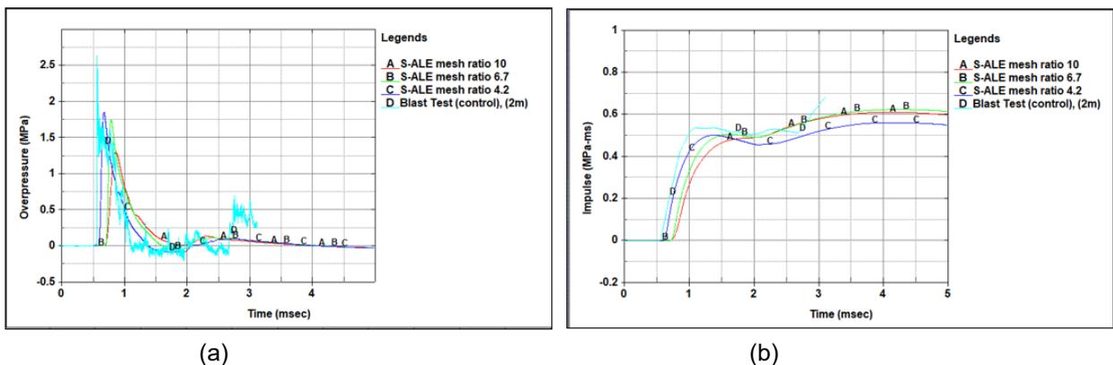
Figure 5: Comparison of various mesh sizes with blast test result, (a)the incident pressure and (b)incident impulse time history at 2m from TNT charge.
