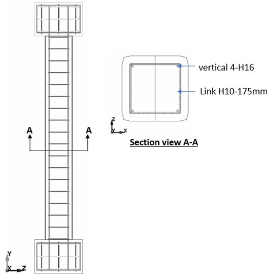
Figure 1: RC beam-column rebar details
