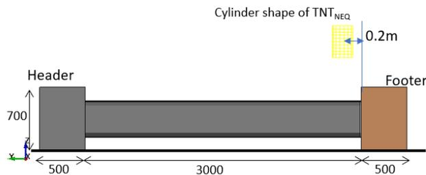
Figure 3: RC Beam-Column blast model setup
