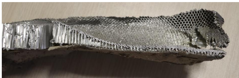
Fig. 1: Honeycomb after high velocity plate impact
