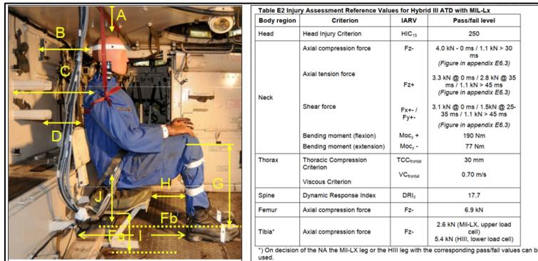
Fig.4: AEP-55 STANAG 4569 Allowable dummy loads
