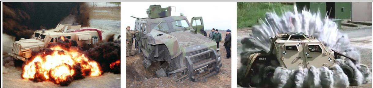
*Fig.1: Military vehicles mine blast tests*
