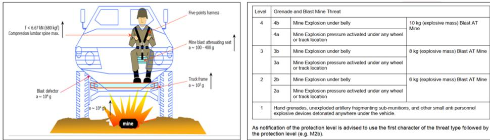
Fig.3: Mine explosion levels
