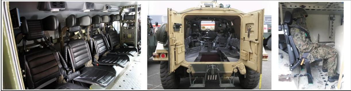
Fig.2: Armoured vehicle personnel compartment
