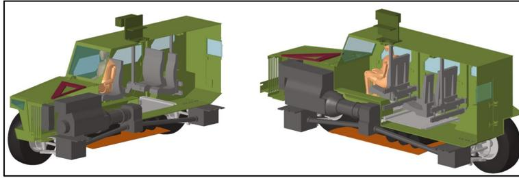
Fig.8: 4x4 military vehicle section view
