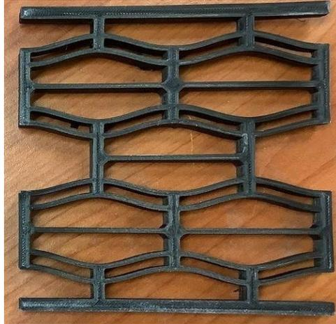
Fig.2: Example of Negative Stiffness Honeycomb structure
