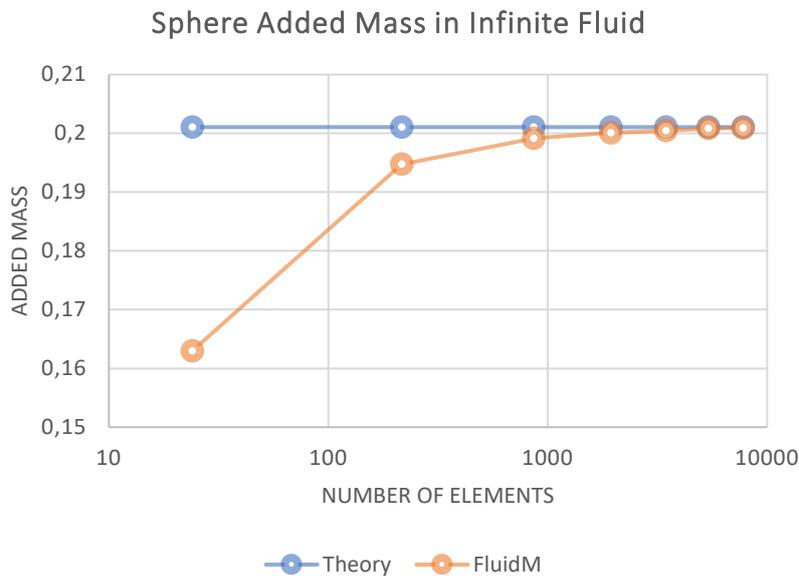
Fig.2: Sphere added mass in infinite fluid.
