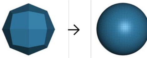
Fig.1: Sphere model with coarse and refined meshes.
