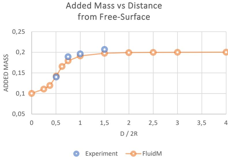
Fig.3: Sphere added mass in fluid with free surface.
