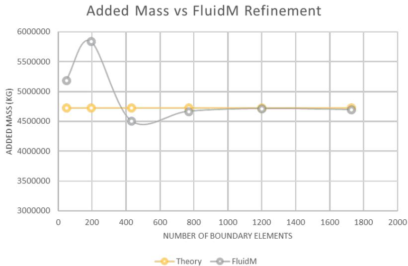
Fig.6: Added mass vs fluidM boundary element mesh.
