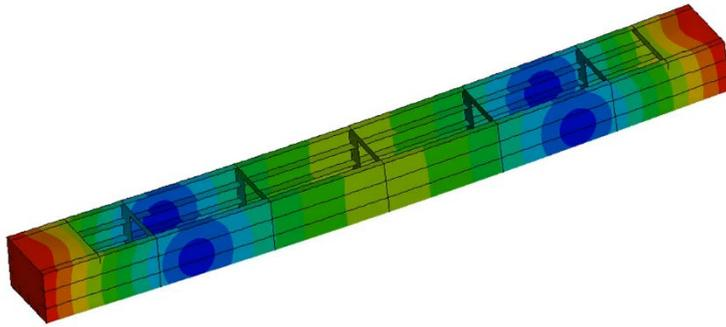
Fig.17: in-fluid mode 9 (1<sup>st</sup> vertical bending)
