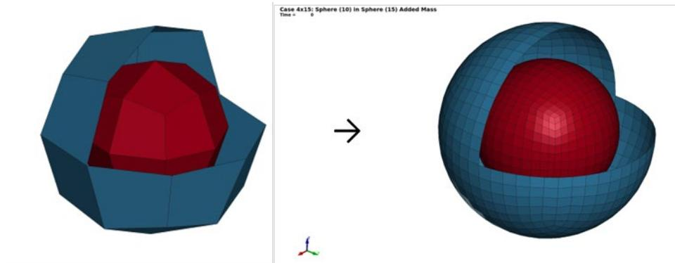
Fig.5: Refinement of the boundary element mesh (48->1728)
