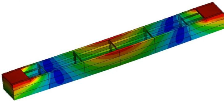
Fig.16: in-fluid mode 8 (1<sup>st</sup> lateral bending)
