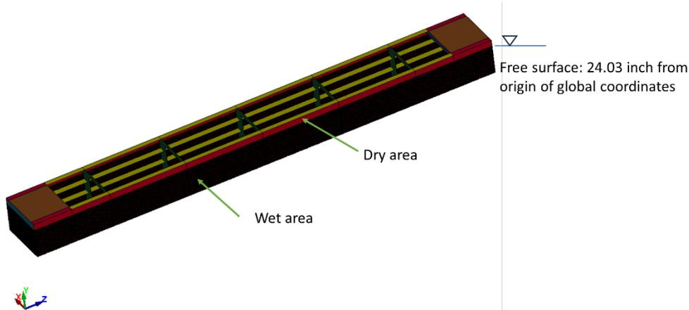
Fig.14: Illustration of wet and dry areas on the box exterior
