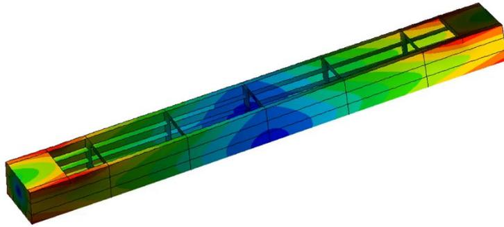
Fig.15: In-fluid mode 7 (1<sup>st</sup> torsion)
