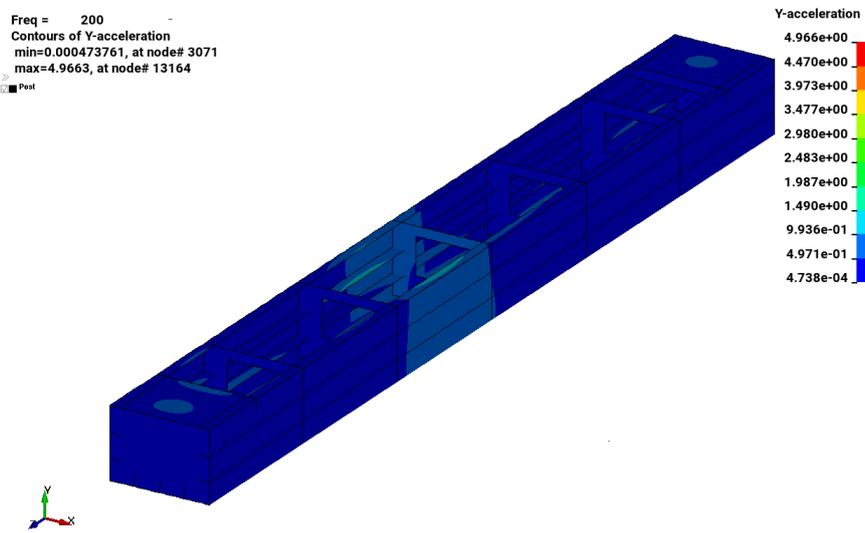
Fig.20: Amplitude of y-acceleration response at 200 Hz (Dry condition)
