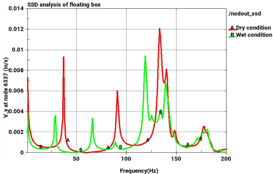
Fig.22: y-directional velocity in dry and wet condition
