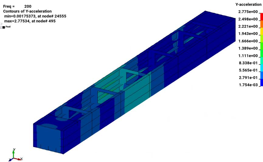
Fig.21: Amplitude of y-acceleration response at 200 Hz (Wet condition)
