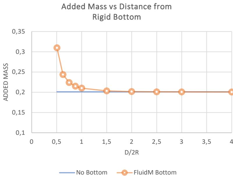
Fig.4: Sphere added mass in fluid with a rigid bottom.
