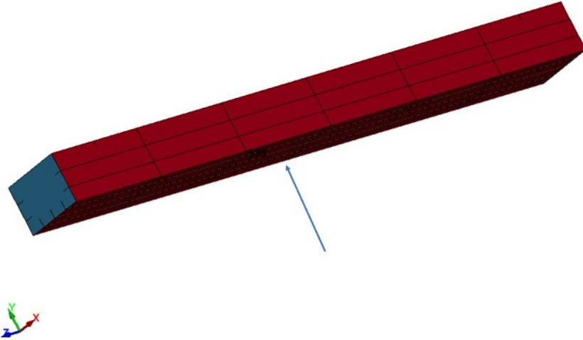
Fig.19: Harmonic Nodal force applied to the bottom of the floating box.
