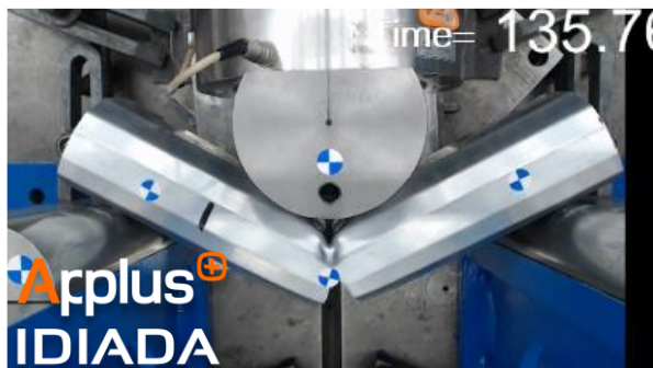
CAE correlation quasi-static 3-point bending tests using SAMP-1. Courtesy of Faraday Future
