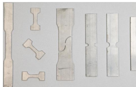
Coupon specimens. Courtesy of Faraday Future
