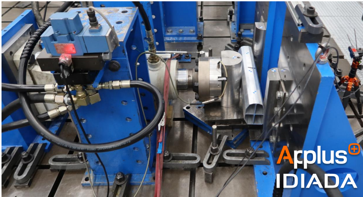
Component test setup for quasi-static 3-point bending tests. Courtesy of Faraday Future
