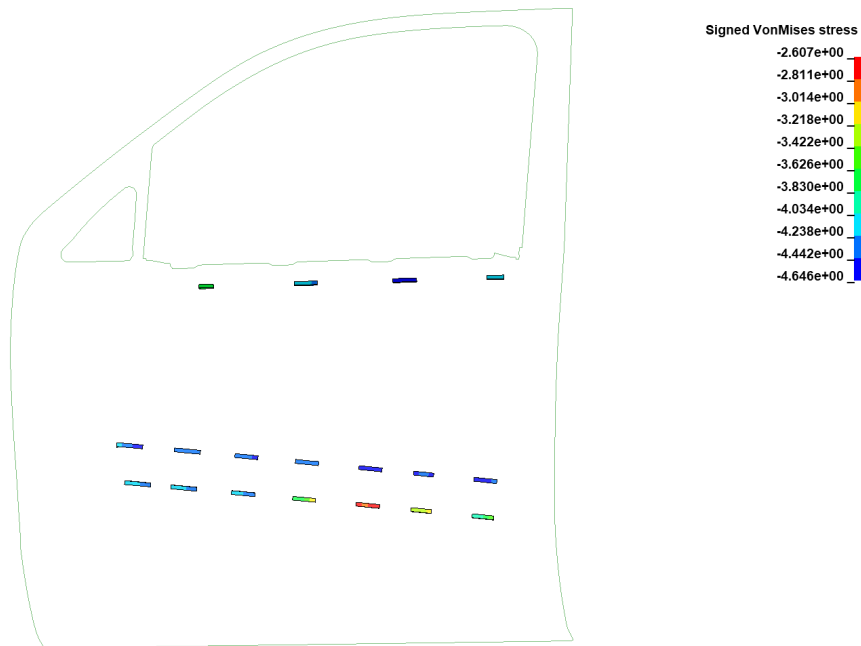
Fig.8: Signed Von-Mises stress contour for the antiflutter beads
