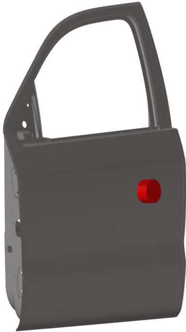
Fig.2: Indenter placement in relation to the Chevrolet Silverado door
