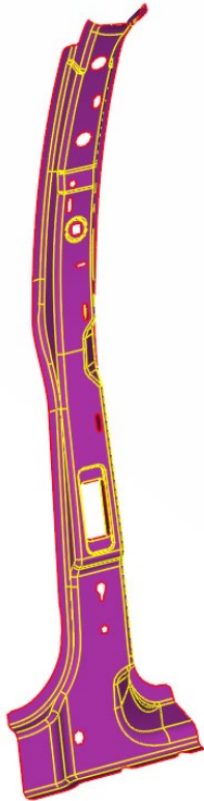
Fig.4: B – pillar with complex perimeters
