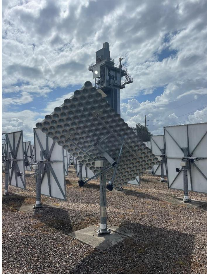
Fig.2: A field trial of the new dimple mirror panel at a test site of the Commonwealth Scientific Industrial Research Organisation in Australia.
