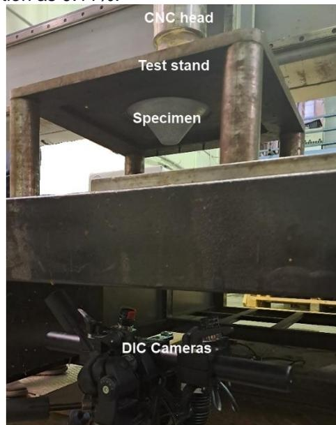
Fig.7: DIC strain measurement setup.
