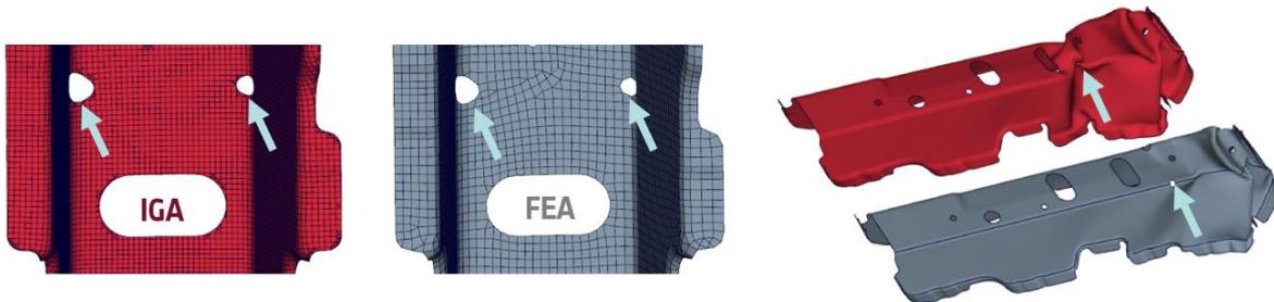
Fig. 16: Seat cross-member: Comparison of the deformation behavior governed by trigger holes.
