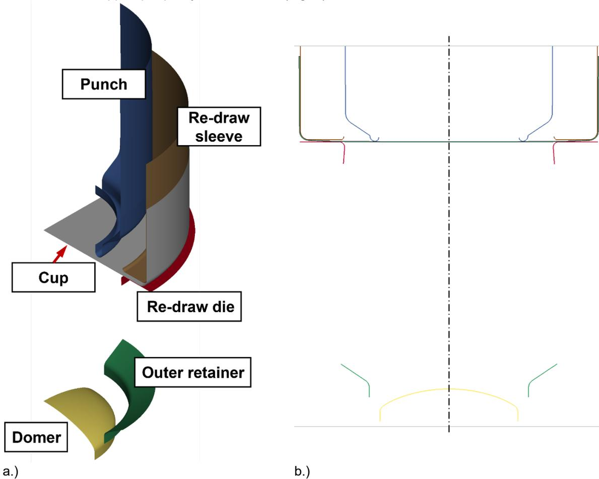
Fig.6: Re-draw and bottom forming tooling, a.) 3D shell model and b.) 2D axisymmetric model.
