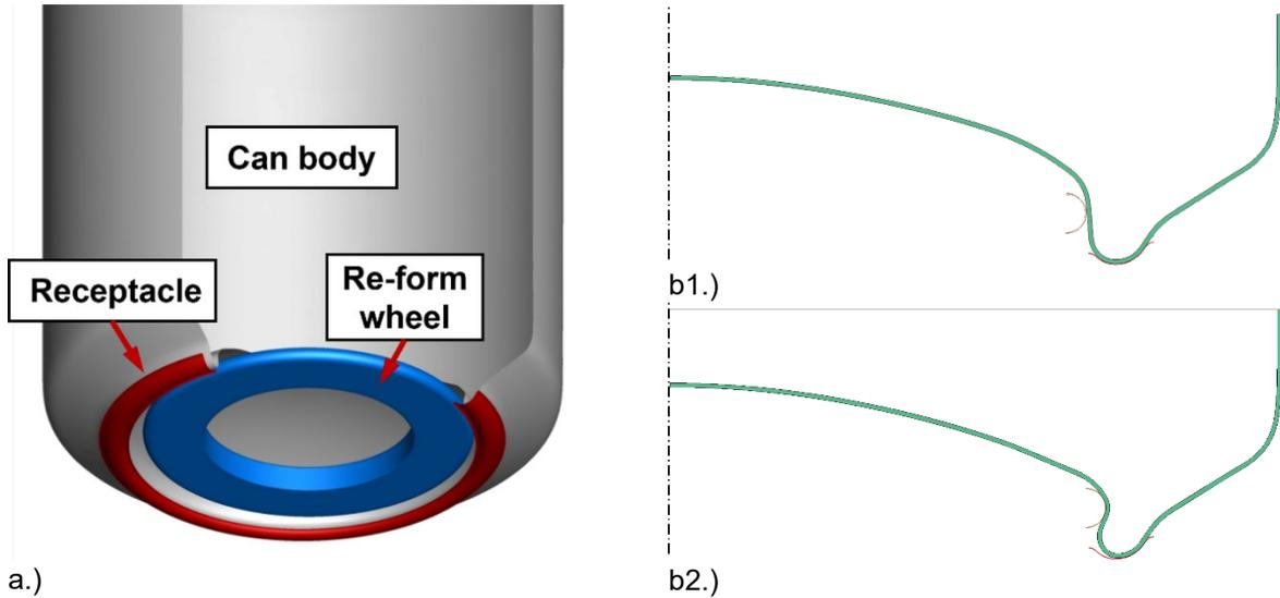
Fig.7: Re-forming operation, a.) 3D shell model, b1.) 2D axisymmetric model initial state and b2.) re-formed state.
