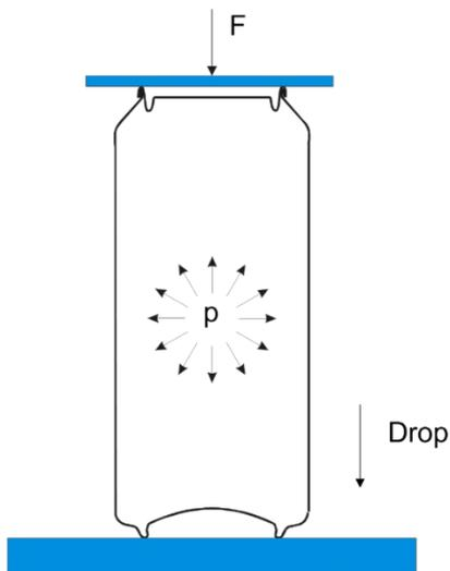
Fig.2: Can body performance testing schematic.
