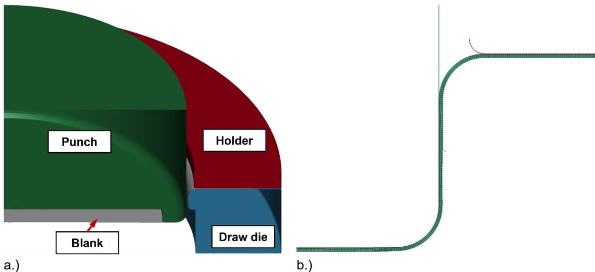
Fig.5: Cup drawing model: a.) 3D shell model and b.) 2D axisymmetric model.
