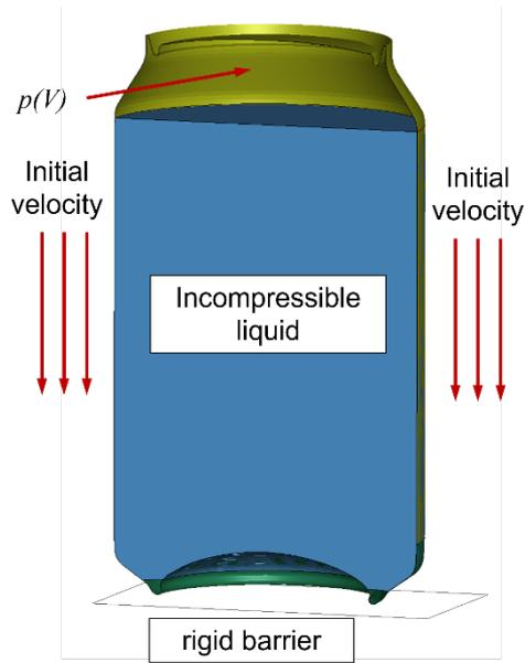
Fig.10: Can body drop model cross-section.
