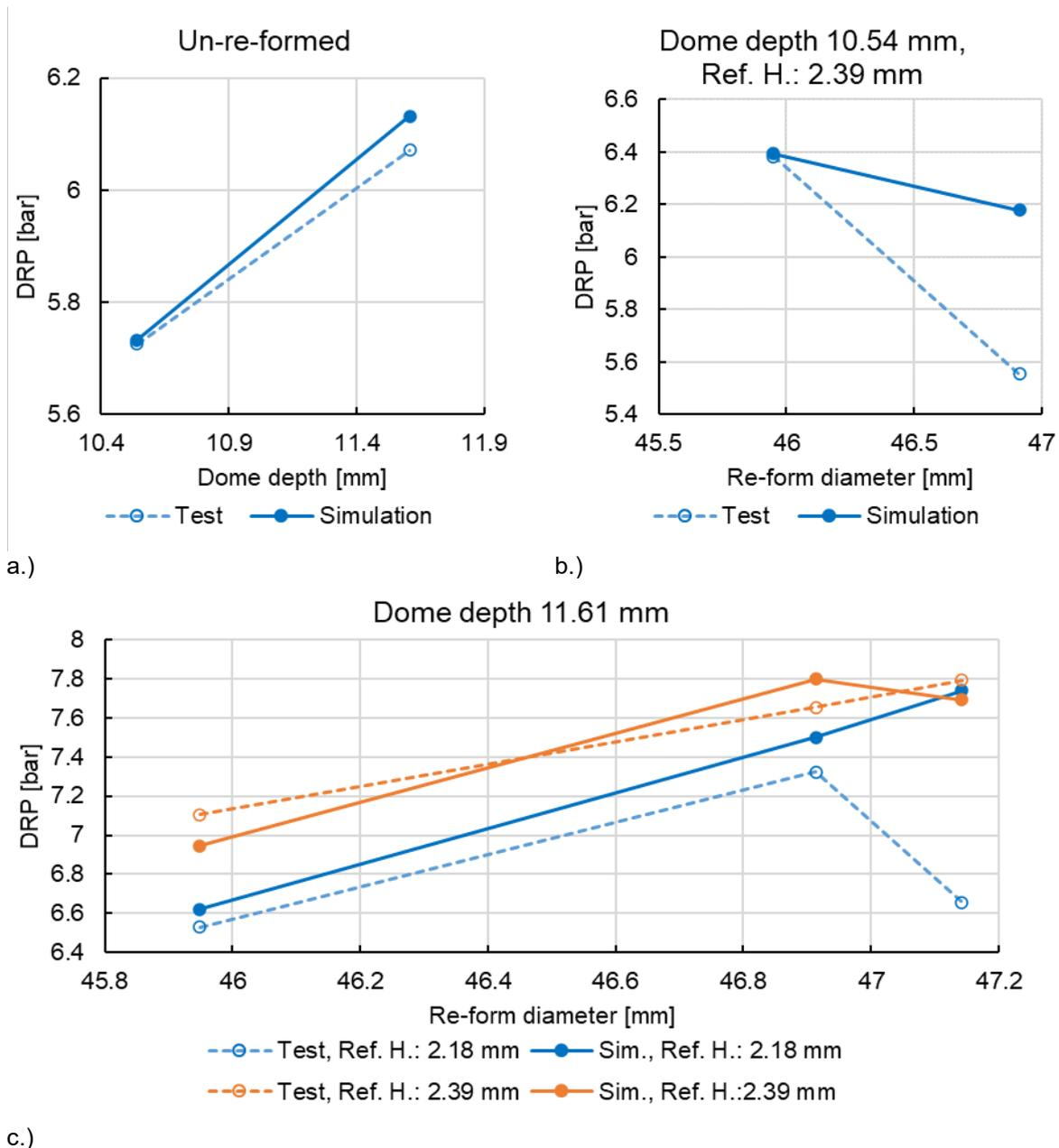
Fig. 12: Dome reversal pressure comparison between test results and simulation predictions: a.) as a function of dome depth of the un-re-formed can body, b.) as a function of re-form diameter, dome depth 10.54mm and re-form height of 2.39 mm, and c.) as a function of re-form diameter at a dome depth of 11.61 mm for two different re-form heights.
