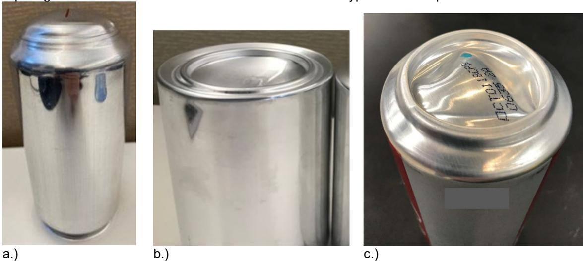
Fig.3: a.) can body after DRP test, b.) can body after axial load exhibiting bottom squat and c.) can body after drop test.
