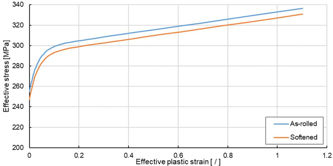
Fig.4: Flow curves of the as-rolled and softened material.
