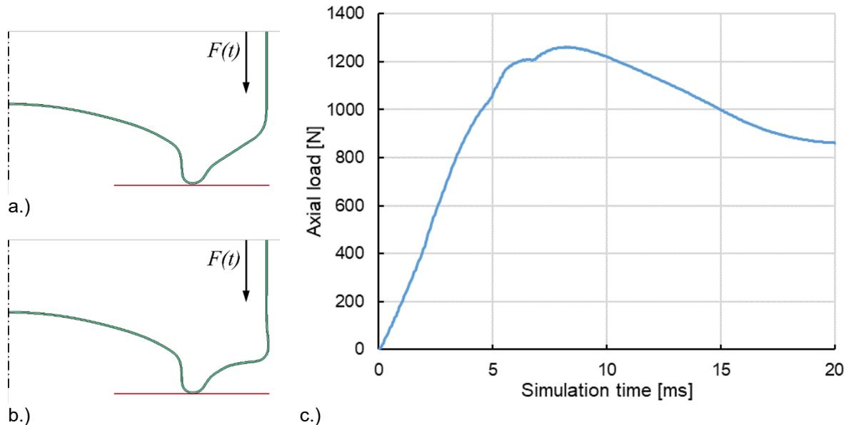
Fig.9: Bottom squat simulation, a.) initial state, b.) deformed can bottom and c.) axial load as a function of simulation time.
