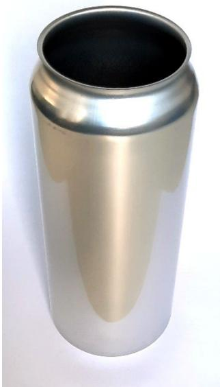
*Fig. 1: Formed blank can body.*
