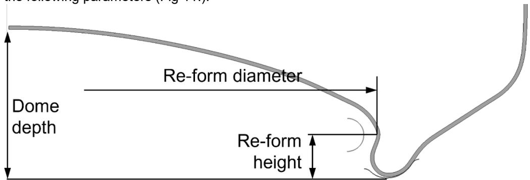
Fig.11: Can bottom geometrical parameters.
