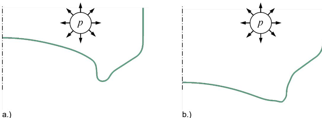
Fig.8: DRP simulation, a.) the initial state of the can body (un-re-formed) and b.) final state of the simulation
