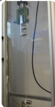
Figure 4.1: Single Dyneema twine tensile test
