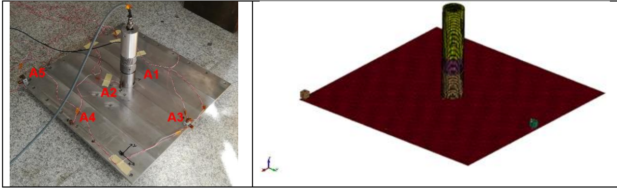
Fig. 9: PSG on a plate experimental set-up, accelerometers locations and associated model
