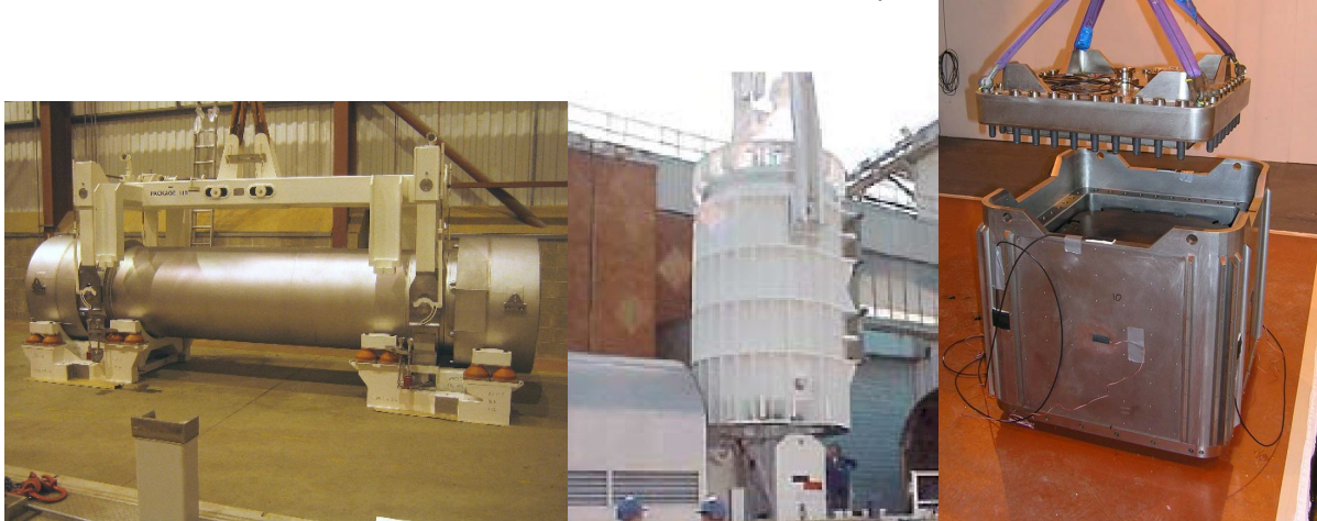
Fig.3: Three forms of shock absorbers
