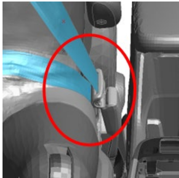
Fig.5: "The seat belt model and pretensioner input model".
