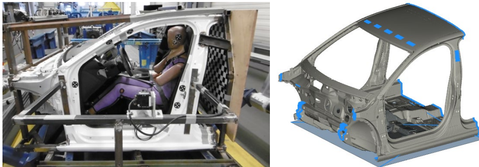
Fig.3: Body fixations on sled / boundary conditions in simulation
