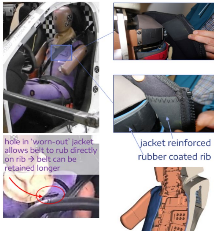
Fig.9: Rubber patches in physical jacket are not present in the FE-model
