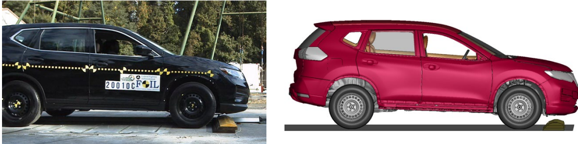
Fig. 10: Suspension test configuration example (a) test; (b) simulation
