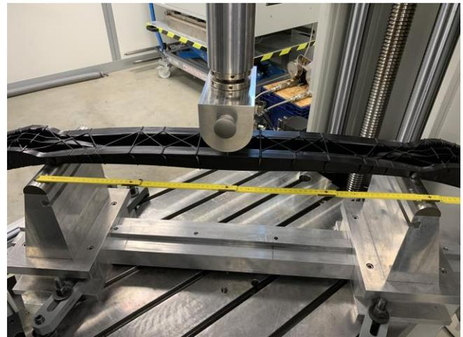
**Figure 4a:** The front bumper beam model made from TAFNEX™ CF-PP-UD-Tapes and back-injection molded with PP-LGF30.
