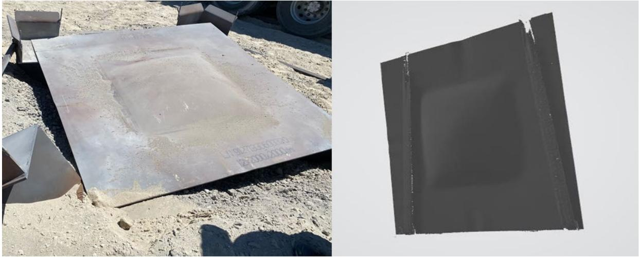
*Fig. 4 Deformed armoured plate and scanned data*
