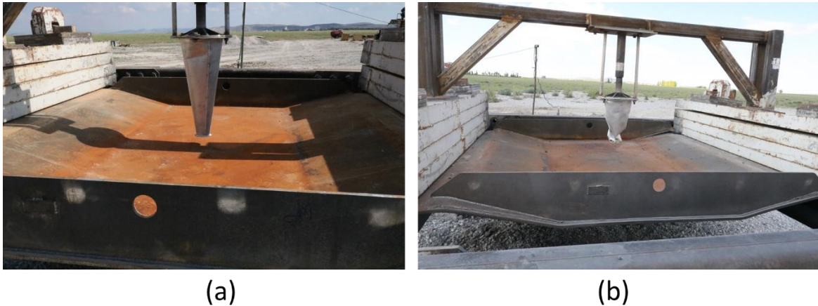
Fig.12: Twisted plate test (a) Before test (b) After test
