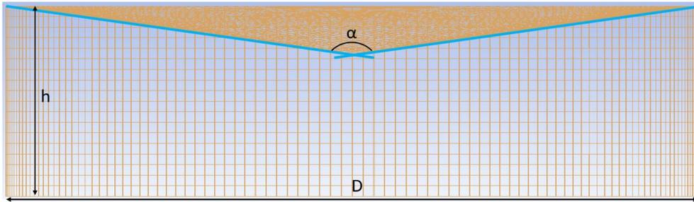
Fig.4: Explosive shape (mesh view).
