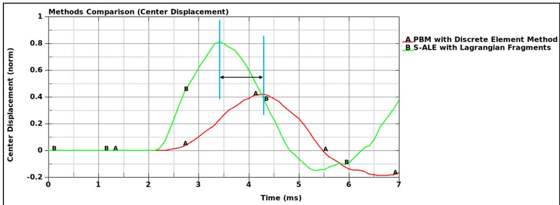
Fig. 16: Center displacement comparison between methods.
