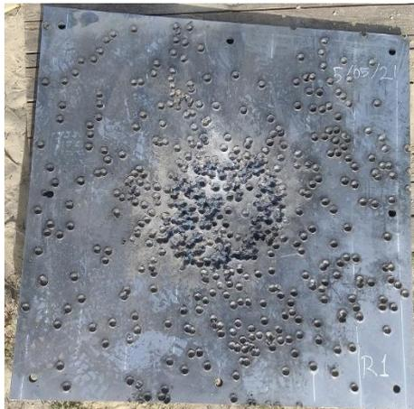
Fig. 15: Fragment dispersion on target plate.
