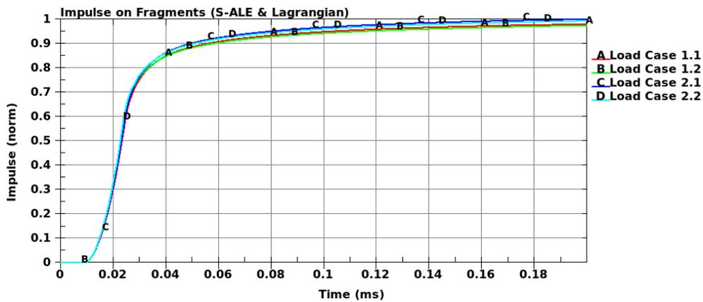
Fig.12: Impulse on fragments (S-ALE & Lagrangian)
