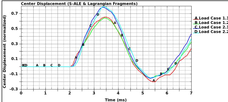
Fig. 14: Center displacement (normalized) of target plate.
