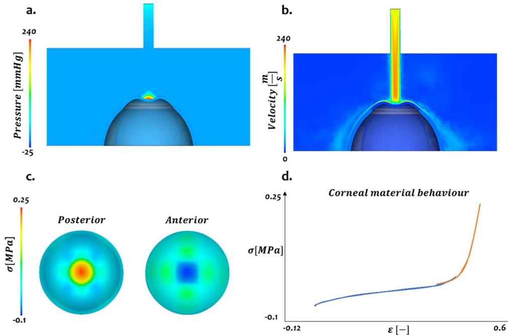
Figure 4: NCT results: a. air pressure and b. air velocity contours at the instant of highest concavity. c. First principal stress distribution in the anterior and posterior surfaces at the instant of highest concavity. d. Corneal material behaviour during the NCT simulation, the red line indicates tension state and the blue line compression state.
