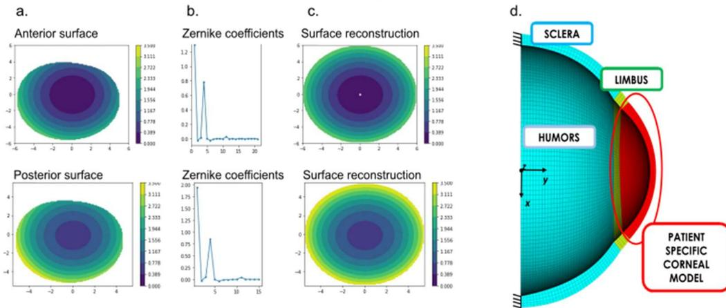
Figure 1: a) Elevation data from *Pentacam* for the anterior and posterior surfaces of the cornea. b) Zernike coefficients found to adjust the *Pentacam* data. c) Reconstructed patient-specific corneal surfaces. d) Structural model of the eye.
