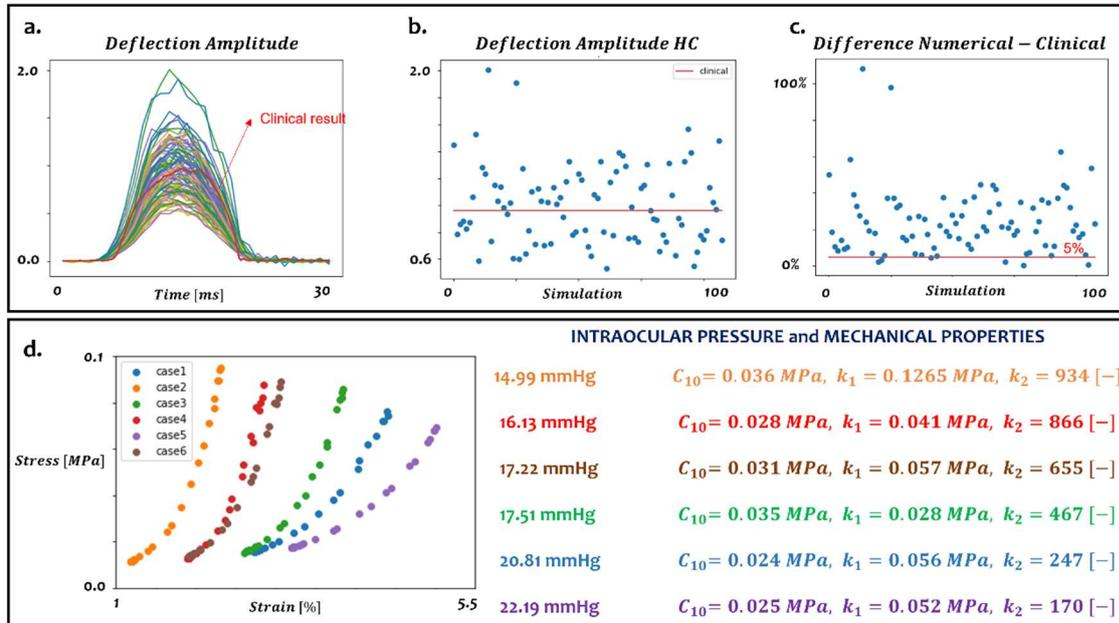
Figure 5: Results of the Montecarlo simulation. a. Deflection amplitude computed for each simulation, b. Value of the deflection amplitude at highest concavity (HC). c. Percentage difference between the numerical deflection amplitude at HC and the clinical deflection amplitude at HC. d. Analysis of the mechanical properties of the corneal tissue and of the IOP for the cases where the difference in the deflection amplitude is lower than 5%.
