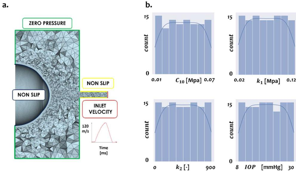
Figure 3: a. Fluid domain of the FSI simulation. b. Corneal material parameter and IOP used in the Montecarlo simulation. Count indicates the number of simulations in which each parameters assumed a value in a certain range.
