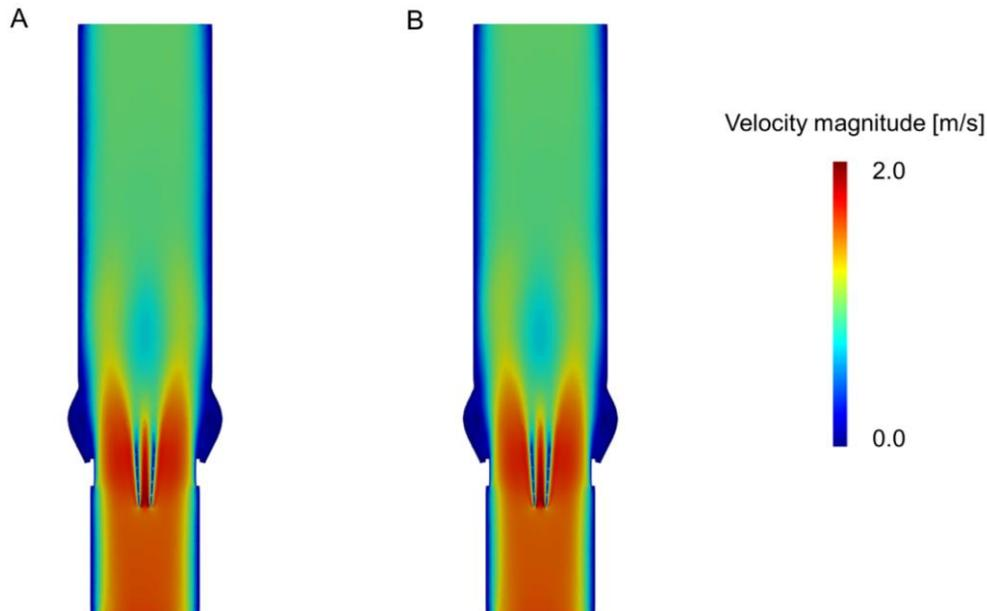
Fig.8: Velocity magnitude in the fluid domain on a long-axis section at  $t = 1.6$  s for the simulations without gap closure treatment (A) and with `*ICFD_CONTROL_GAP` (B).
