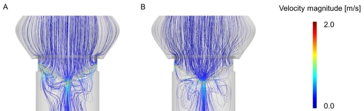
Fig.7: Streamlines at  $t = 1.2$  s for the simulations without gap closure treatment (A) and with `*ICFD_CONTROL_GAP` (B).
