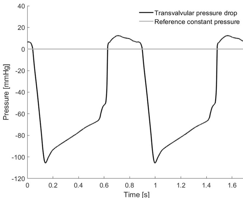
Fig.3: Pressure waveforms applied as boundary conditions: reference constant pressure (outlet) and transvalvular pressure drop (inlet).
