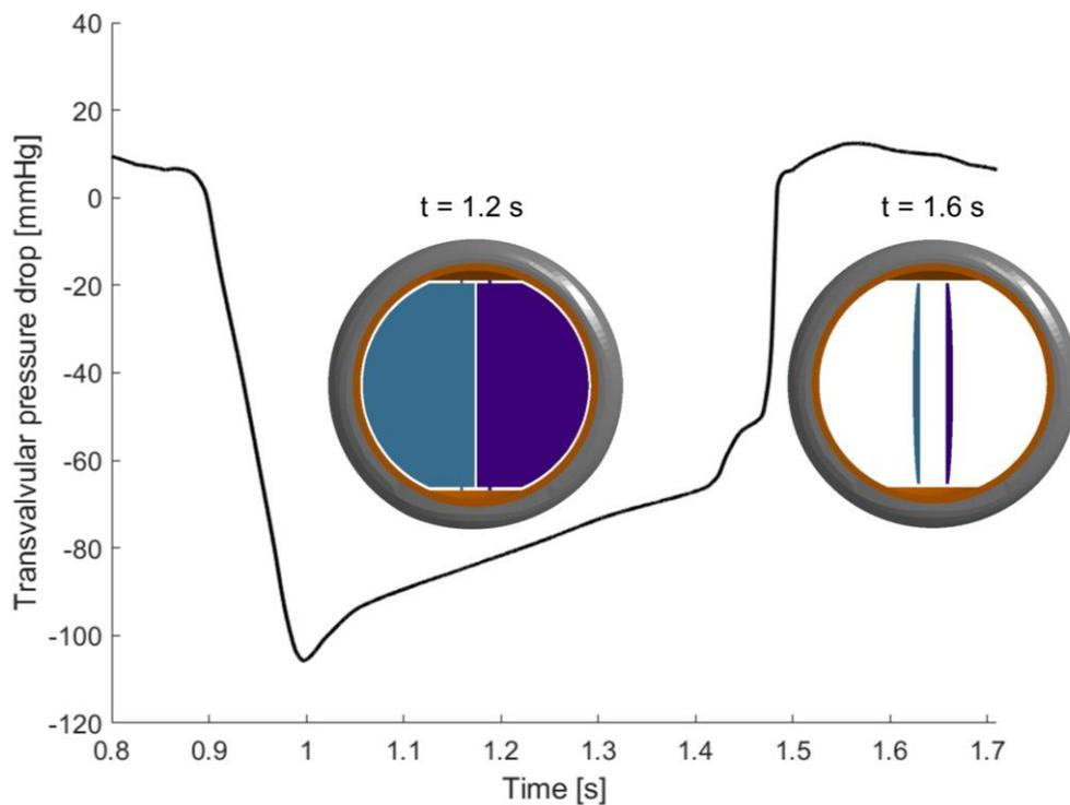
Fig.4: Closed and open configuration of the valve at mid-diastole and mid-systole.
