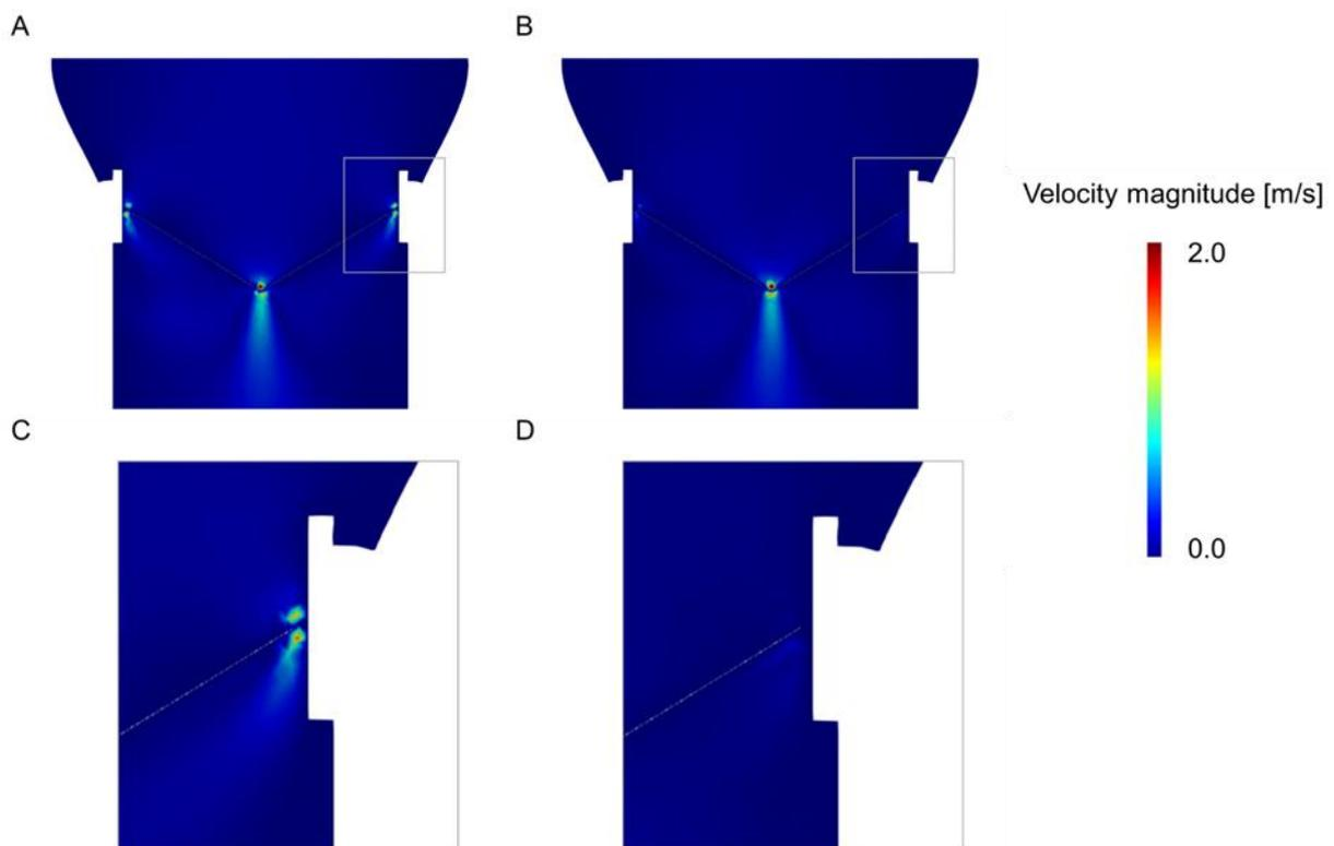
Fig.6: Velocity magnitude in the fluid domain on a long-axis section at  $t = 1.2$  s for the simulations without gap closure treatment (A, C) and with `*ICFD_CONTROL_GAP` (B, D).
