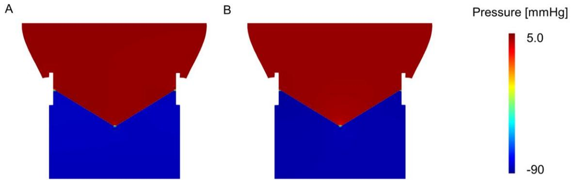
Fig.5: Pressure in the fluid domain on a long-axis section at  $t = 1.2$  s for the simulations without gap closure treatment (A) and with `*ICFD_CONTROL_GAP` (B).
