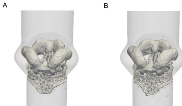
Fig.9: Isosurfaces depicting swirling strength in the valve region at  $t = 1.6$  s for the simulations without gap closure treatment (A) and with `*ICFD_CONTROL_GAP` (B).
