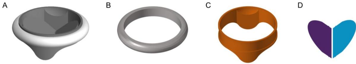
Fig.1: CAD model of the mechanical aortic valve (A) and its different components: sewing cuff (B), housing (C) and leaflets (D).
