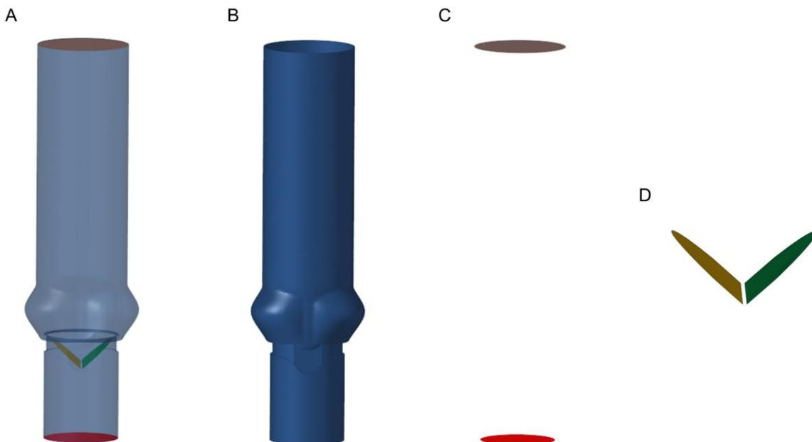
Fig.2: Fluid domain (A) and its different components: fluid wall (B), inlet and outlet (C) and fluid leaflets (D).
