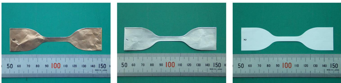
Fig.5: Dumbbell Test Piece Anode Collector (Left), Cathode Collector (Center) and Separator (Right)
