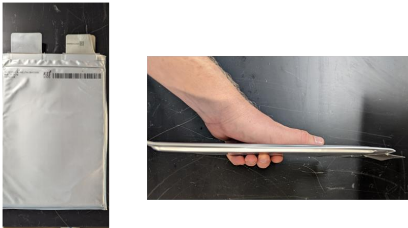
Fig.2: Pouch cell used for the Ansys experiments (Ansys test cell)
