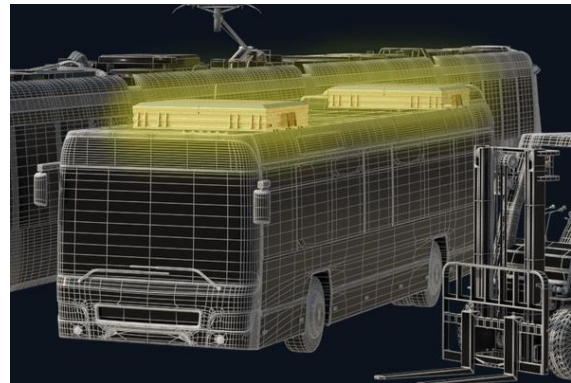
Fig. 1: a) FE Model of battery pack, b) public transport bus traction battery placement.
