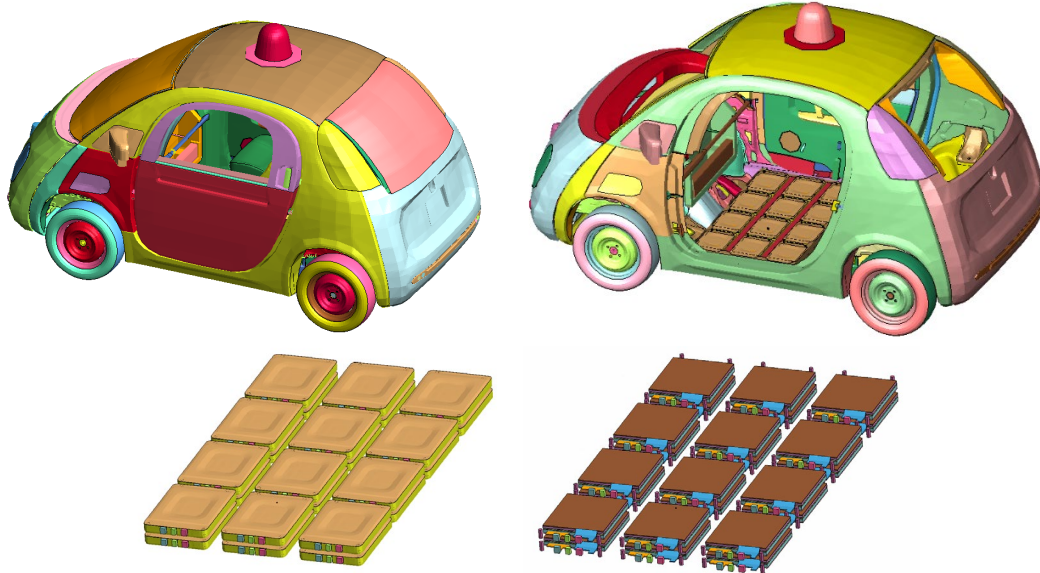
Figure 3 EV Model (Top Left), Battery Pack in EV Model (Top Right), 24 Battery Modules (Bottom Left), Internal Structure of Battery Module (Bottom Right).
