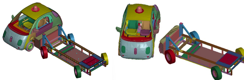
Figure 6 MDB Side Impact Model (Left) and Simulation Result (Right)
