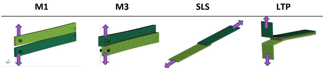
Fig.1: Numerical models for the four selected specimen types
