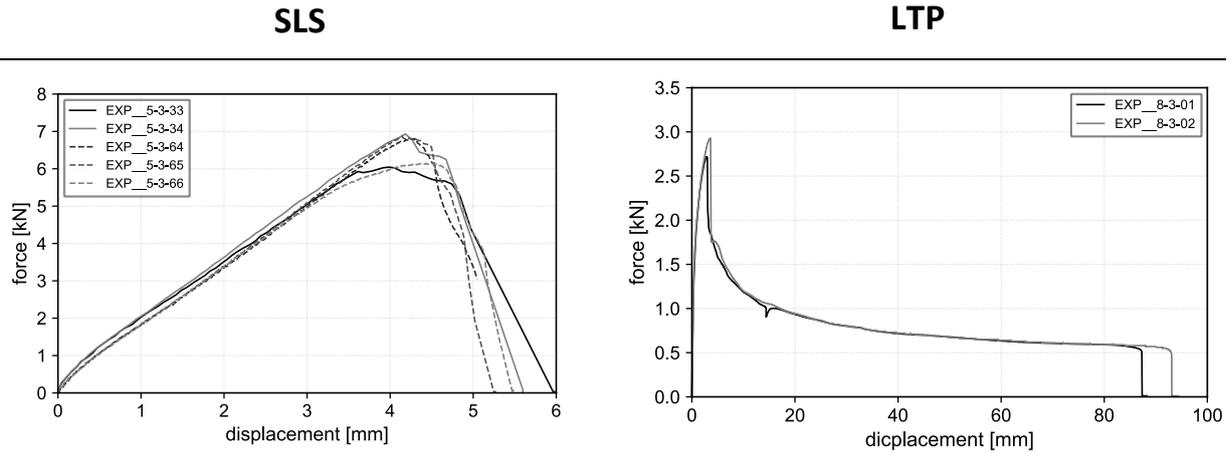
Fig.3: Experimental test curves for SLS and LTP tests
