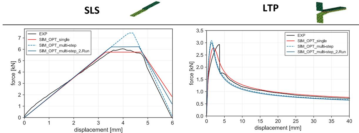
Fig.8: Force-displacement curves of the optimized material card based on the fracture mechanics and coupon tests
