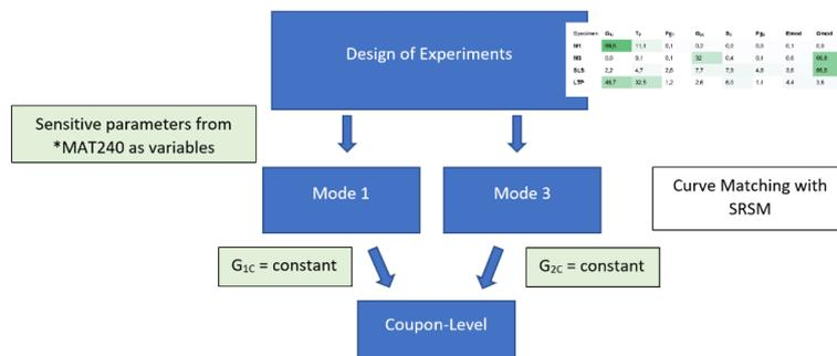
Fig. 5: LS-OPT workflow for the optimization of material parameters for \*MAT\_240
