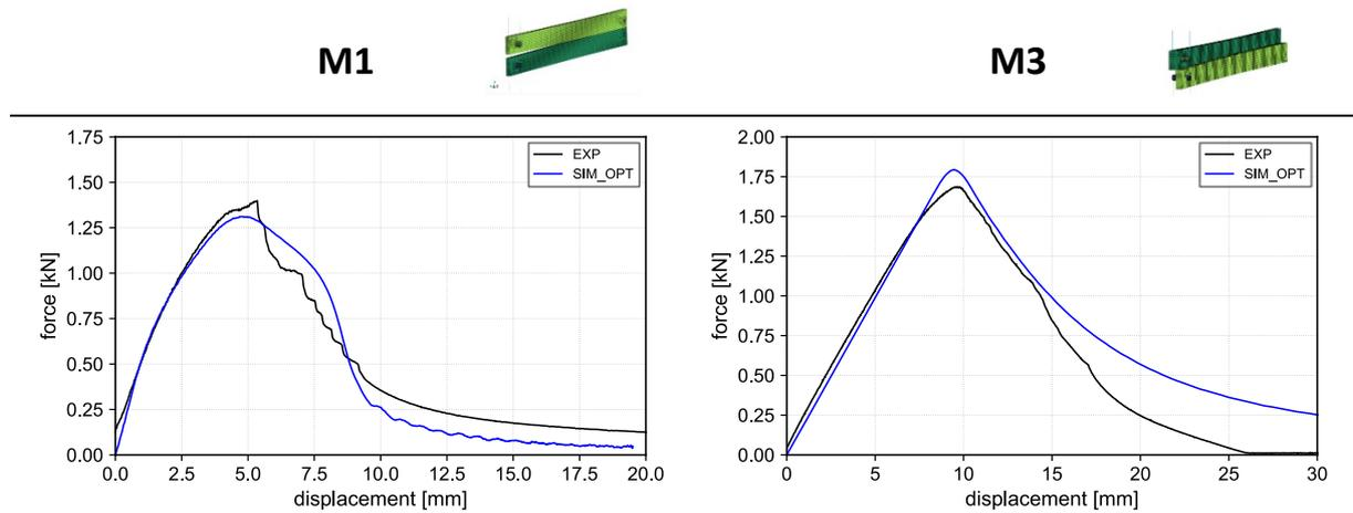
Fig.7: Force-displacement curves of the optimized material card for the fracture mechanical tests
