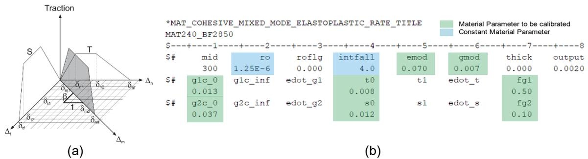
Fig.4: Mixed-mode traction-separation law of **\*MAT\_240** (a) [1] and an example of material card **\*MAT\_240** for an adhesive layer (b)
