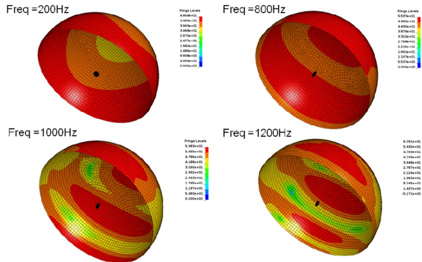
**Figure 6: Sound pressure level contours of field points**
