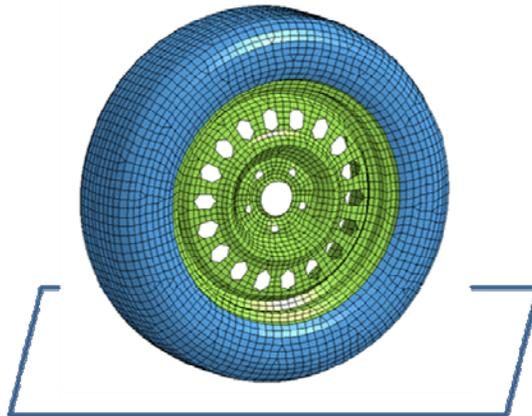
**Figure 5: Reflecting surface was modeled as rigid**
