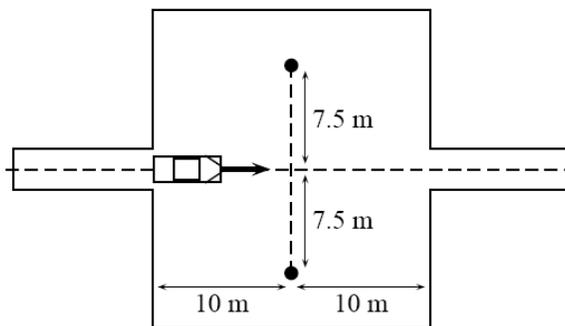
**Figure 3: the setup for a pass-by noise test form the ISO 362 Standard.**
