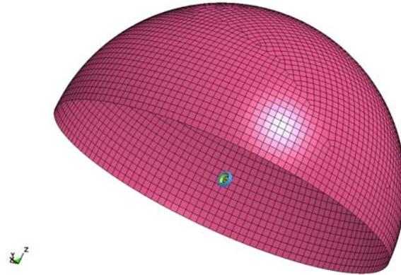
**Figure 4: R7.5 hemi sphere field point used for pass-by noise test**
