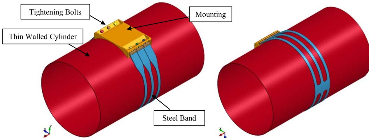
Figure 1: Band clamp assembly model
