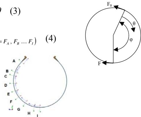
Calculating an average force (Equation 4), shows that the final uniform internal force is equal to the average of the distributed internal forces in the band at the end of the preload stage. This result can be demonstrated in **Figure 15** for  $\mu=1$ .
