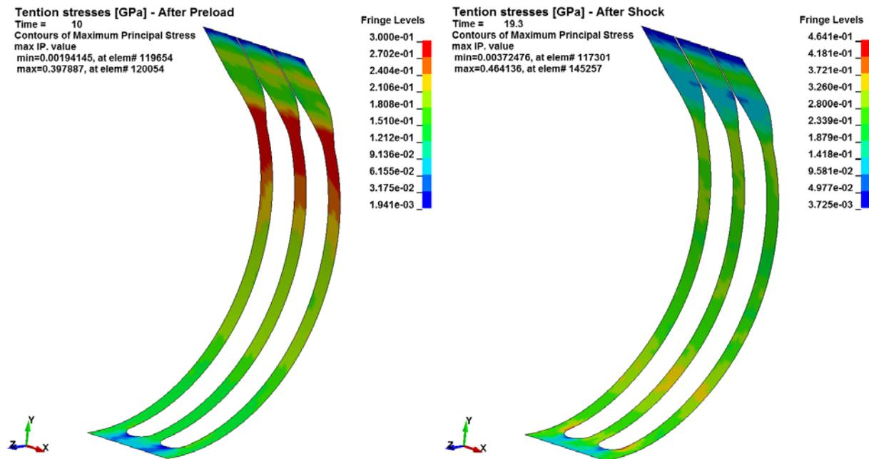
Figure 11: Stress distribution in the band for  $\mu=1$  after preload stage (left) and after the shock (right)
