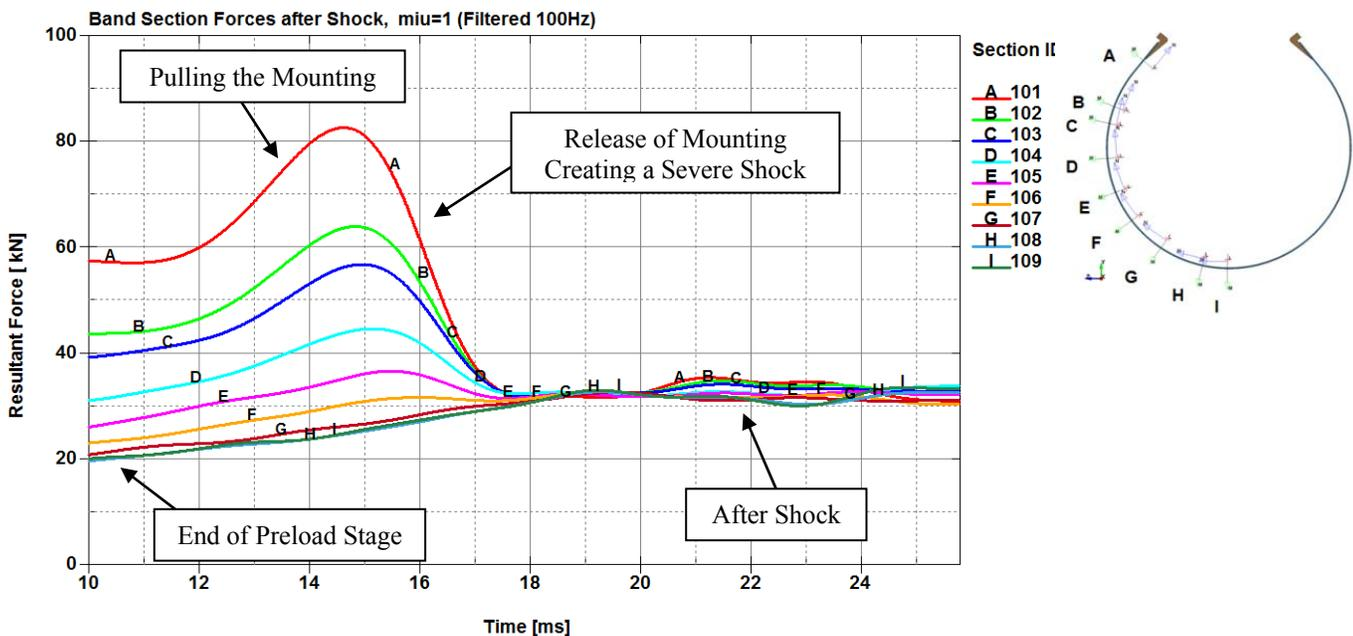
Figure 13: Internal tension forces in the band subjected to severe shock with  $\mu=1$
