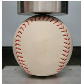
Figure 1. Softball compression test setup.
