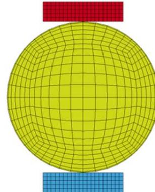
Figure 9. Softball compression test. The bottom (blue) plate is fixed, while the top (red) plate is given a prescribed velocity to compress the ball.
