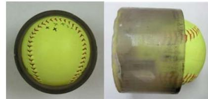
Figure 3. Softball loaded in a ball carrier, or "sabot."
