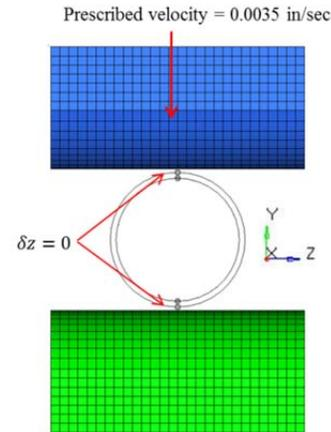
Figure 12. Barrel compression model configuration with boundary conditions (y-z view).
