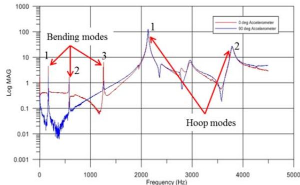
Figure 6. FRF measurement from a hollow baseball bat, displaying three bending modes and two hoop modes [8].
