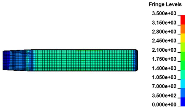
Figure 10. Example von Mises stress fringe plot during the dynamic relaxation pseudo phase for the barrel of the bat. Stress units are psi.
