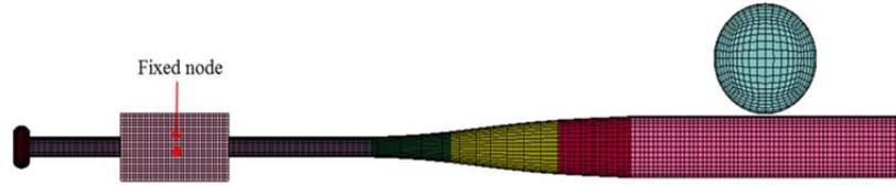
Figure 14. Bat-ball finite element models for a composite softball bat.
