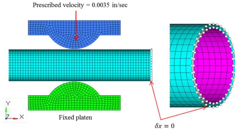
Figure 11. Barrel compression model configuration with boundary conditions (x-y view).
