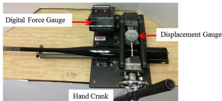
Figure 4. Barrel compression test setup.
