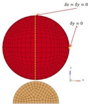
Figure 8. Example CCOR model with boundary conditions.
