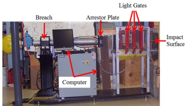
Figure 2. Dynamic stiffness test setup.
