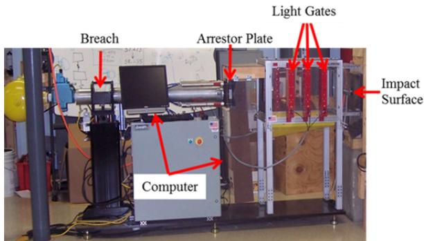
Figure 2. Dynamic stiffness test setup.
