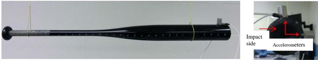
Figure 5. Modal test setup of a simulated free-free condition with accelerometers attached 90° from each other to measure the bending and hoop frequencies of the bat.
