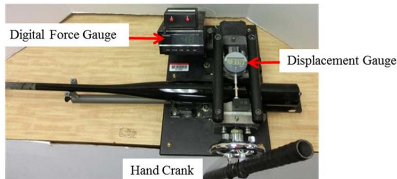
Figure 4. Barrel compression test setup.
