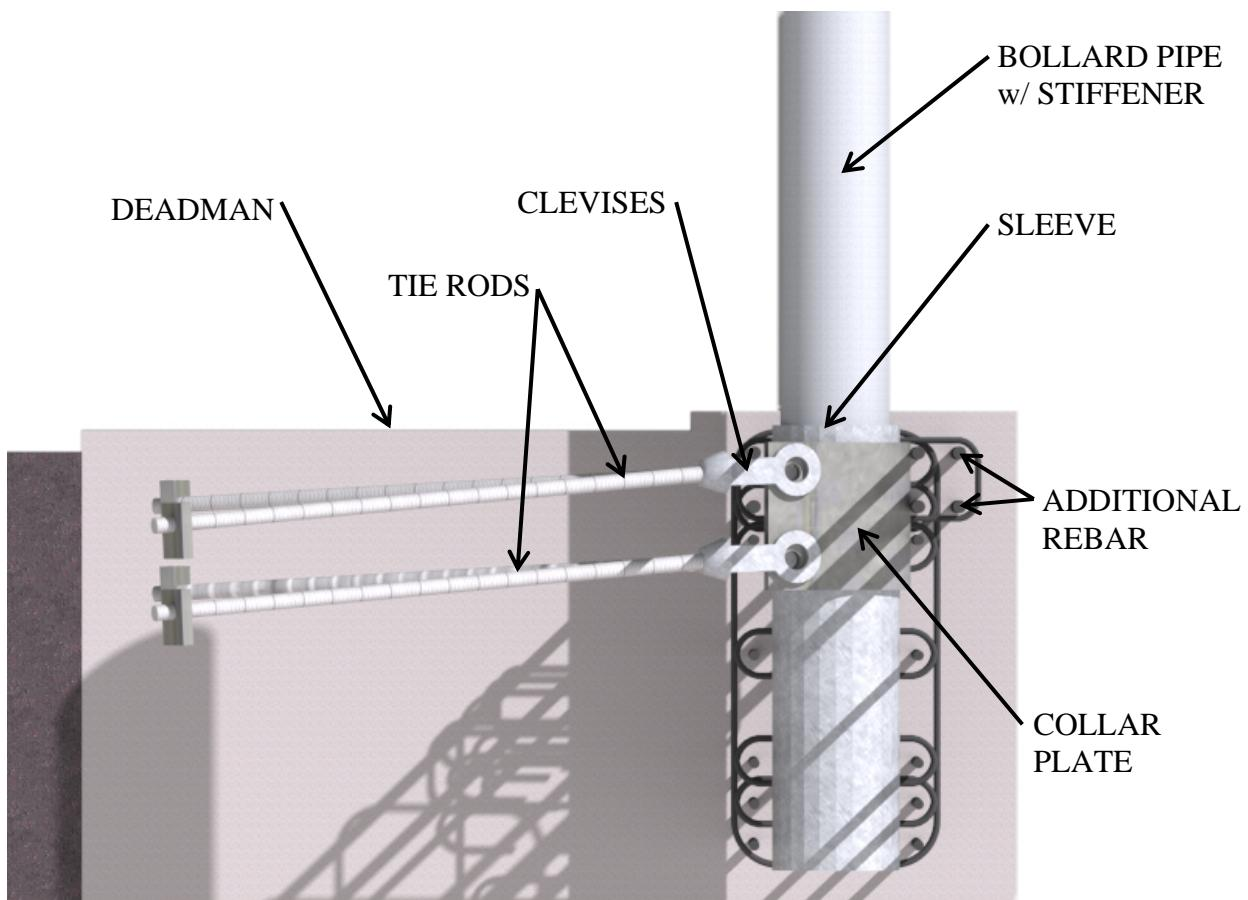
Figure 4 – Section View of Conceptual Subgrade Courtyard Bollard Design
