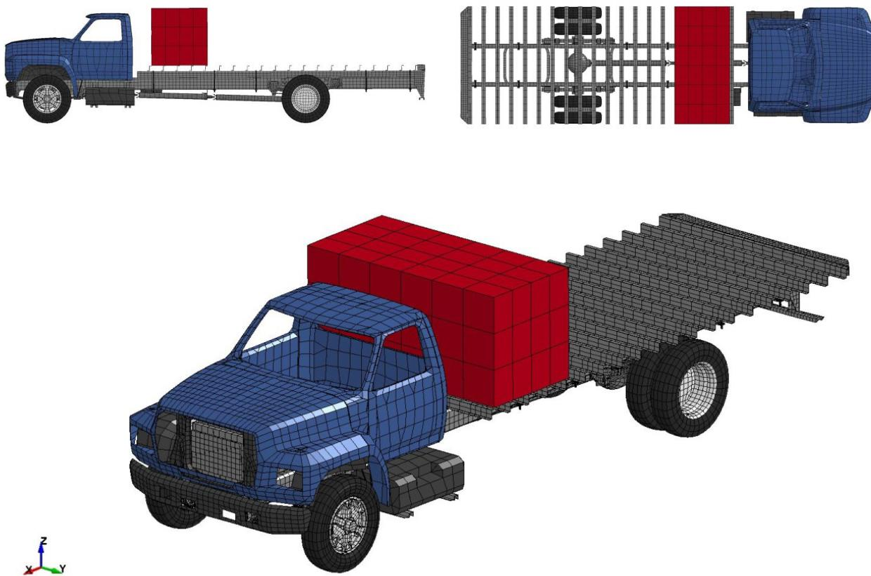
Figure 6 – LS-DYNA K12 (M50) Vehicle Model
