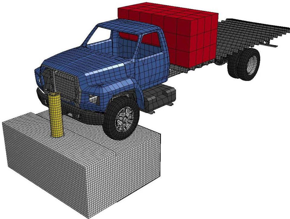
**Figure 7 – LS-DYNA Vehicle Impact Analysis at Initial Time Step**
