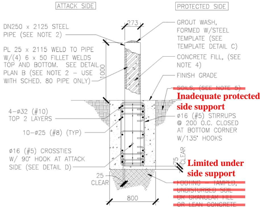
Figure 3 – DoS Standard DS-22 K12 Rated Bollard [3] with Site Specific Considerations
