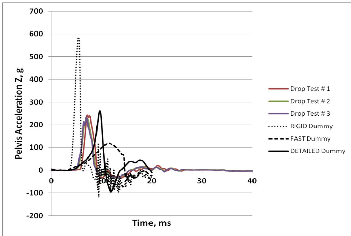
**Figure 9:** Pelvis  $a_z$  test and analysis results
