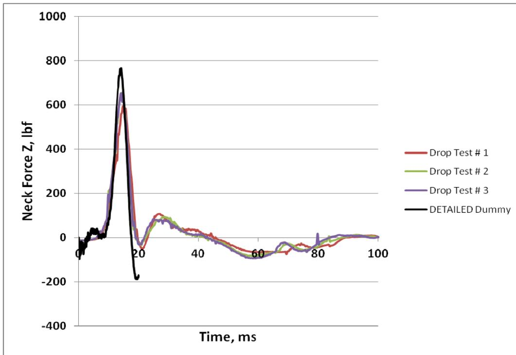
Figure 11: Neck  $F_z$  test and analysis results
