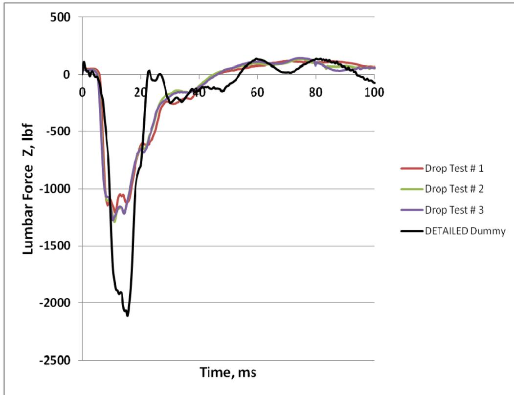
Figure 14: Lumbar  $F_z$  test and analysis results
