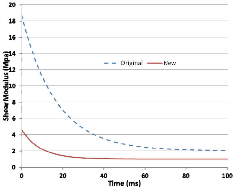
Figure 12: Shear relaxation behavior for lumbar spine material
