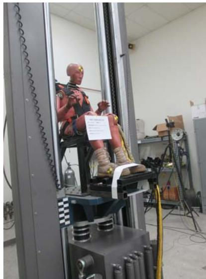
**Figure 2:** Drop tower with Hybrid III 50<sup>th</sup> percentile ATD
