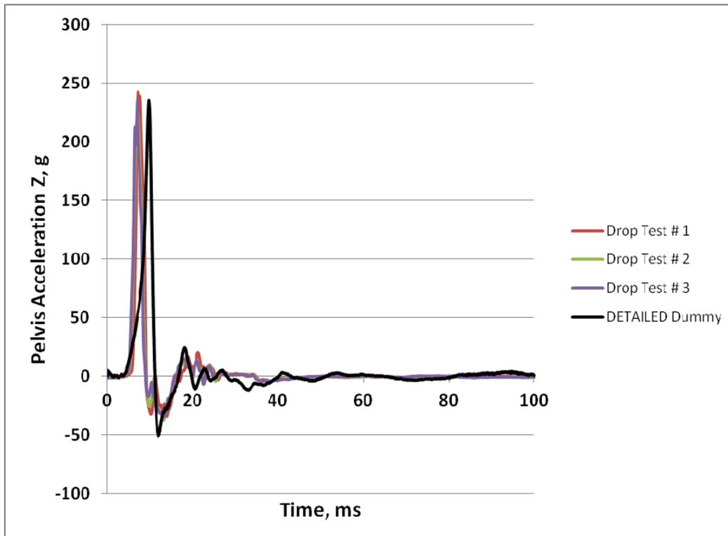
Figure 13: Pelvis  $a_z$  test and analysis results
