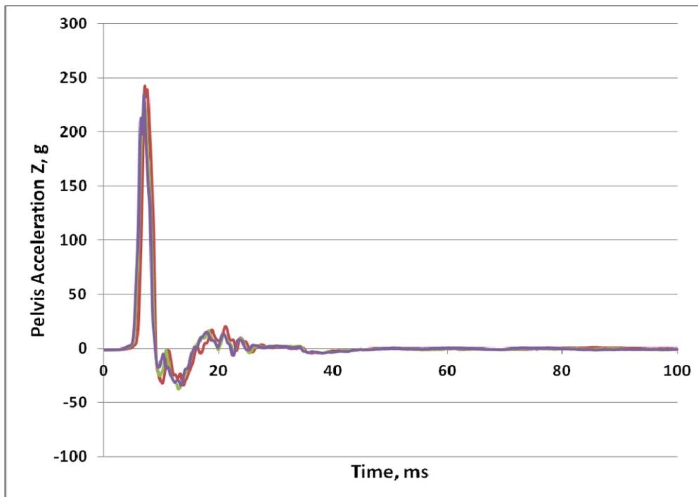
**Figure 6:** Pelvis  $a_z$  test results
