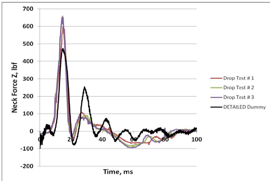
Figure 15: Neck  $F_z$  test and analysis results
