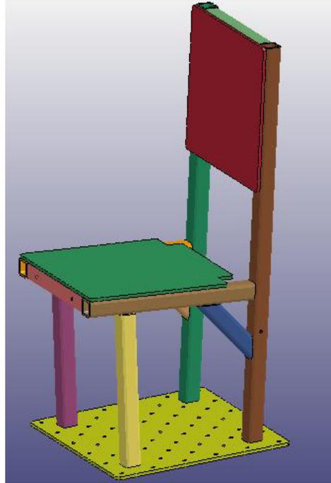
**Figure 7:** Rigid seat finite element model
