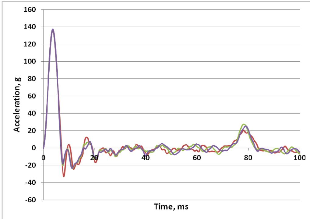
Figure 3: Seat platform acceleration
