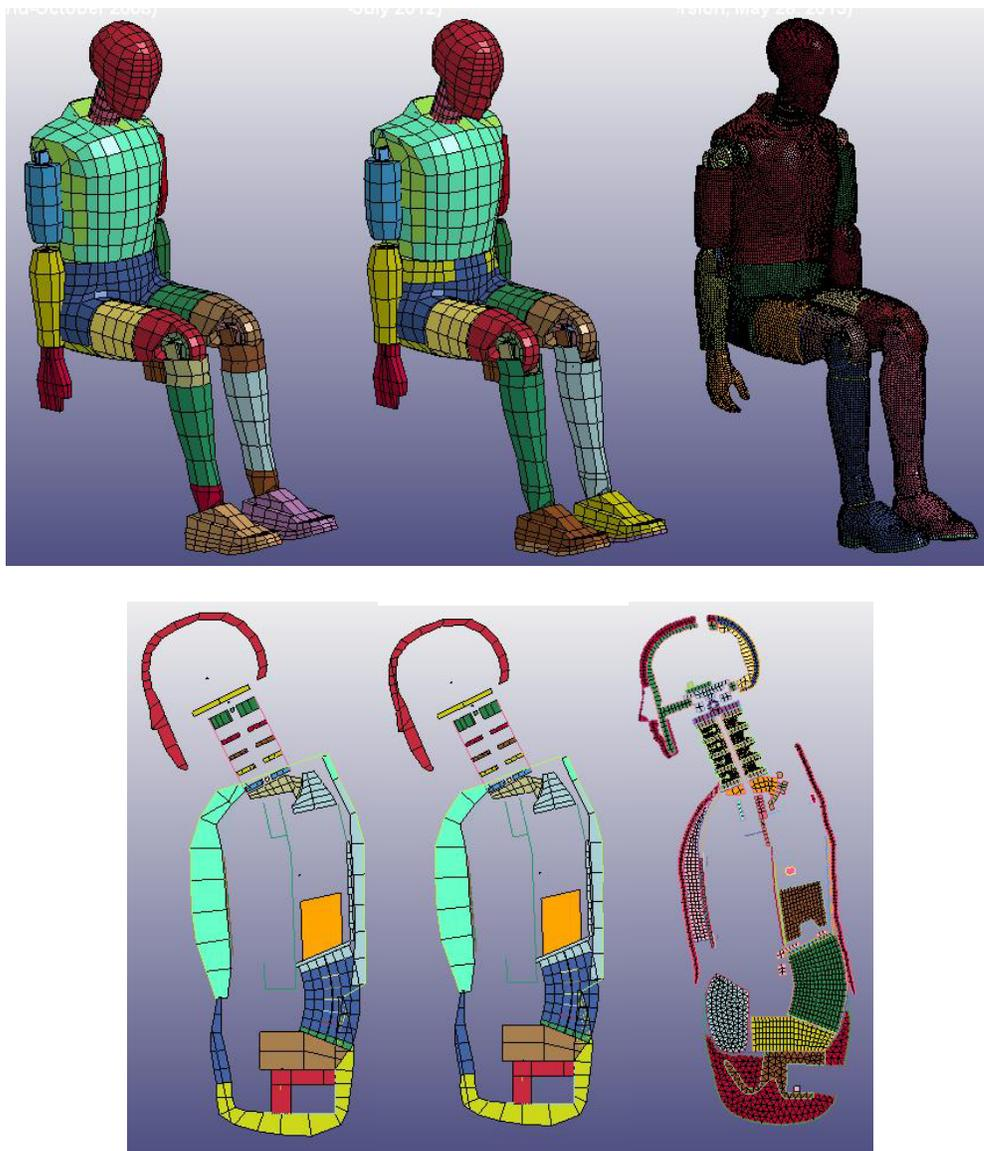
**Figure 1:** RIGID (left) FAST (middle) and DETAILED (right) dummy models
