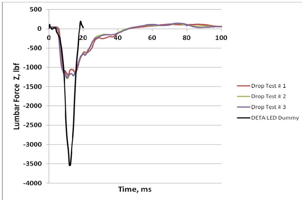
Figure 10: Lumbar  $F_z$  test and analysis results
