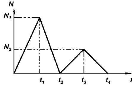
Figure 5. Energy deposition law:  $t_1 = 24 \mu\text{s}$ ,  $t_2 = 49 \mu\text{s}$ ,  $t_3 = 76 \mu\text{s}$ ,  $t_4 = 102 \mu\text{s}$ ,  $N_1 = 9.1 \text{ MW}$ ,  $N_2 = 4.9 \text{ MW}$
