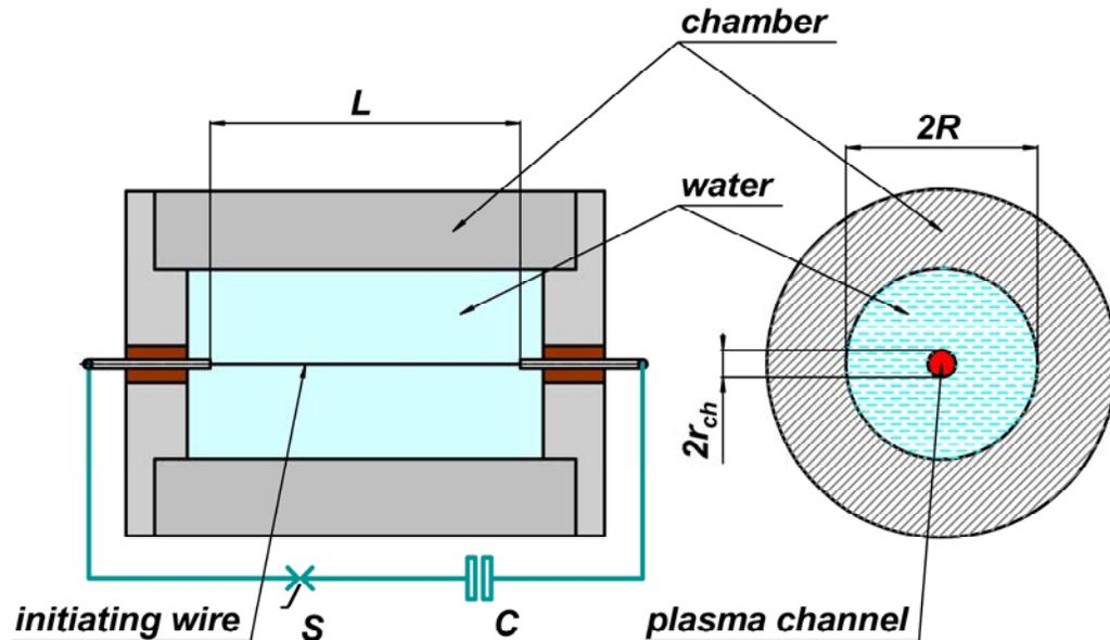
Figure 1. The scheme of the test equipment
