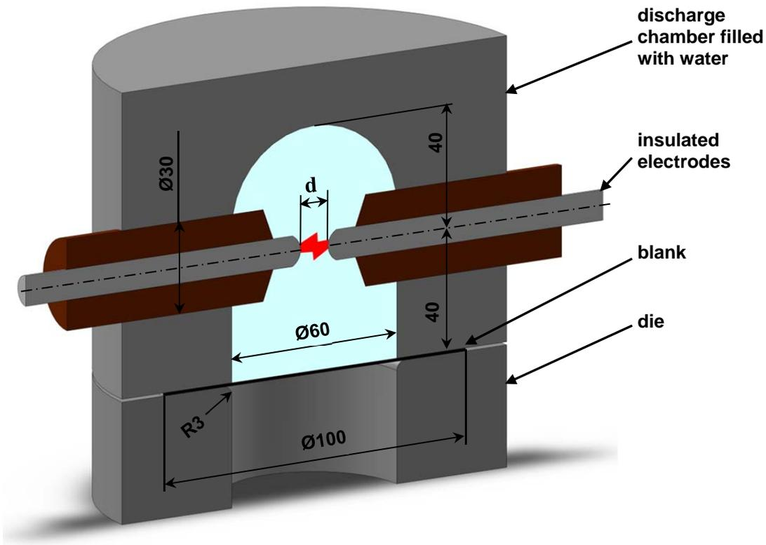
Figure 4. Tool for EHF process
