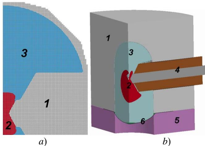
Figure 6. ALE mesh and deformation of the fluid parts and the blank at the moment  $245 \mu\text{s}$
