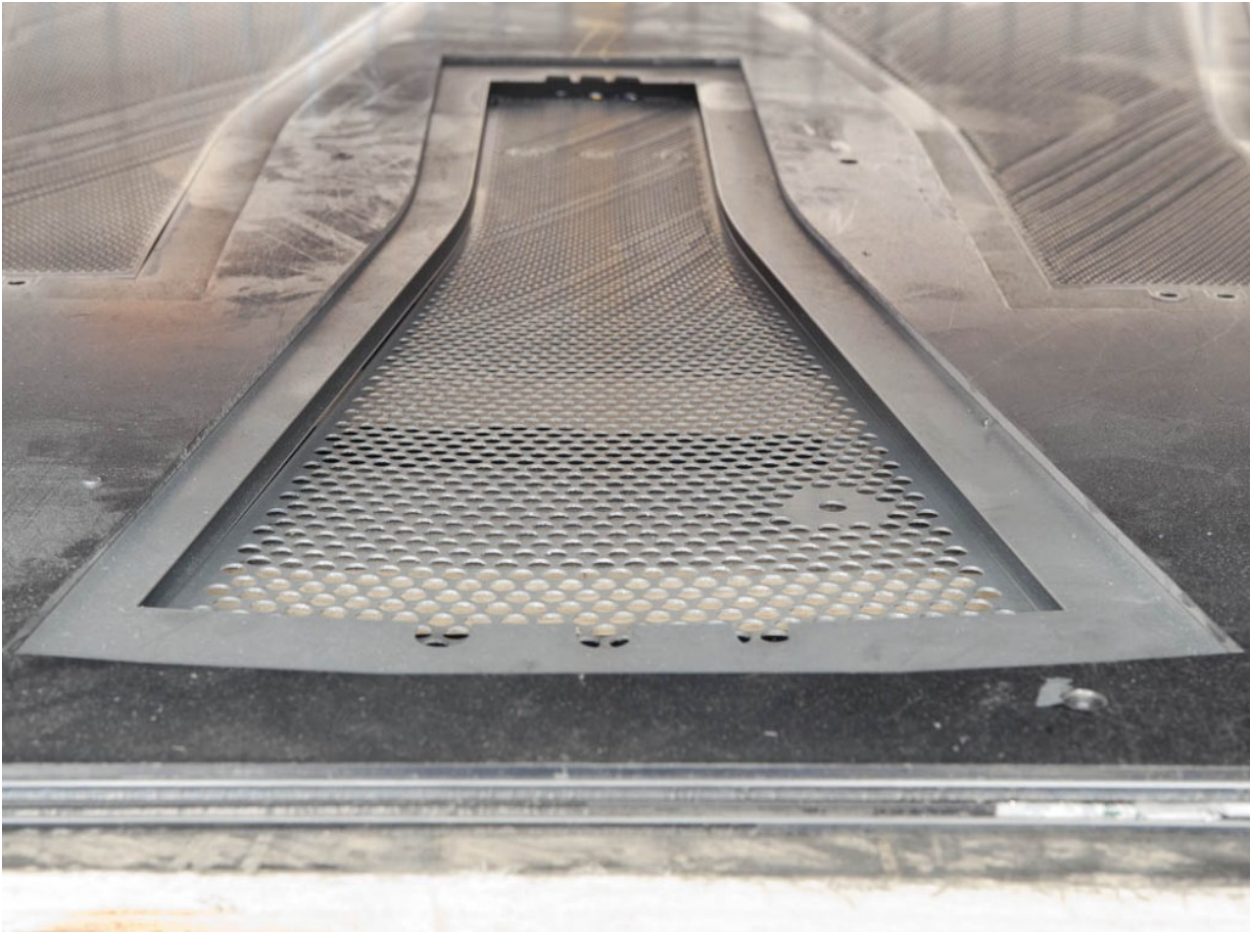
Figure 4 Laser cutting operations to create the outer skin blank
