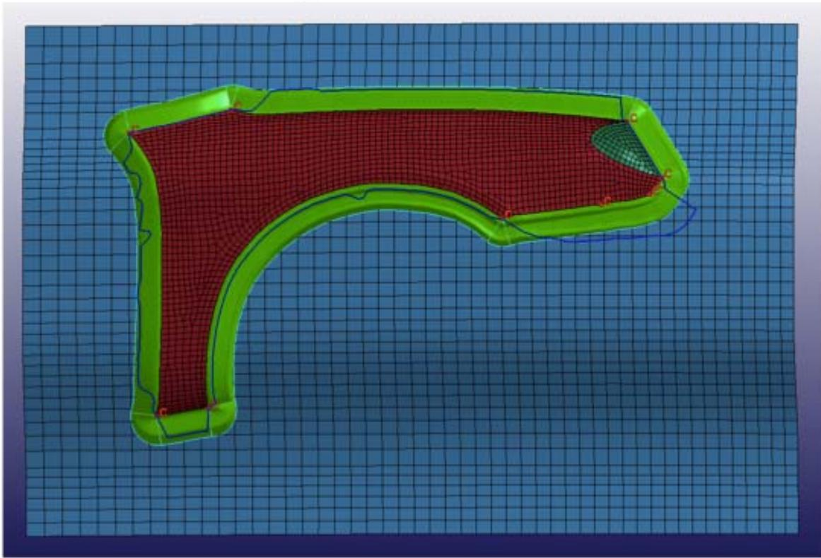
Fig. 7: Addendum with developed flanges shown as blue line
