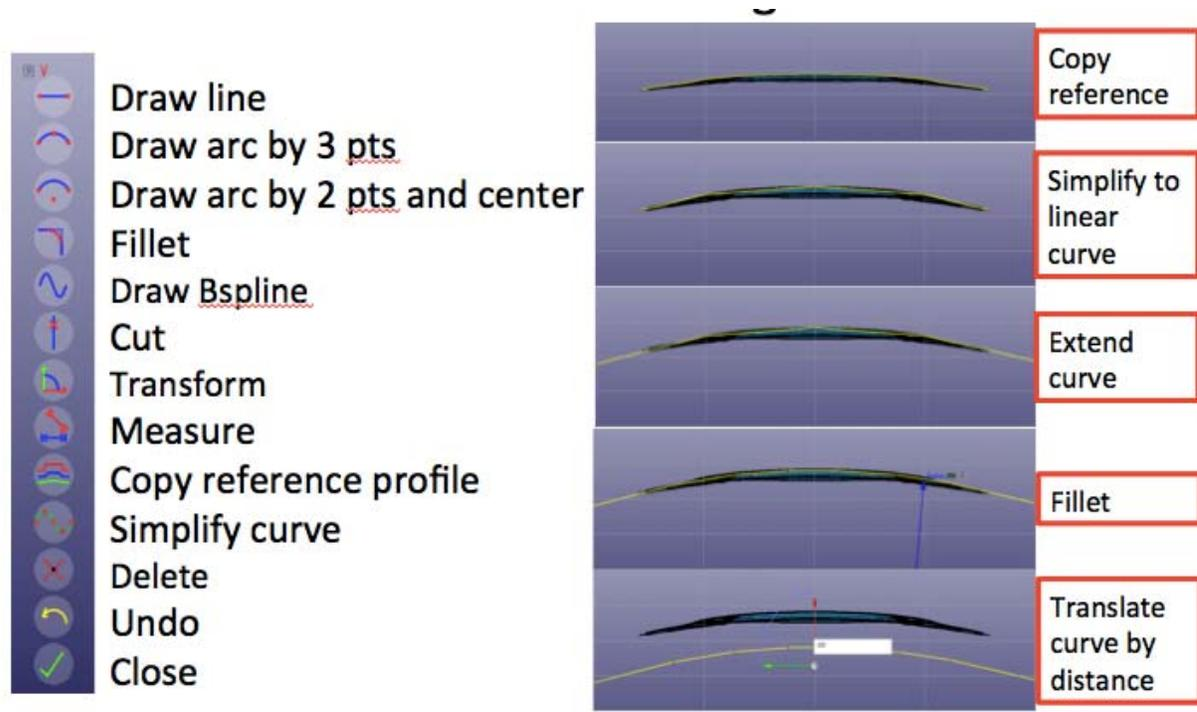
Fig. 4: Functionality to create a binder surface
