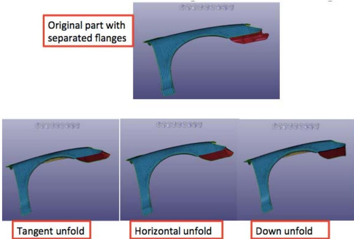
Fig 3: Different unfolding methods (lay out on addendum also possible after addendum is generated)
