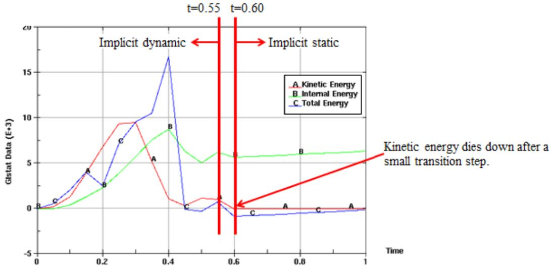
Figure 11. Energy during the switching.
