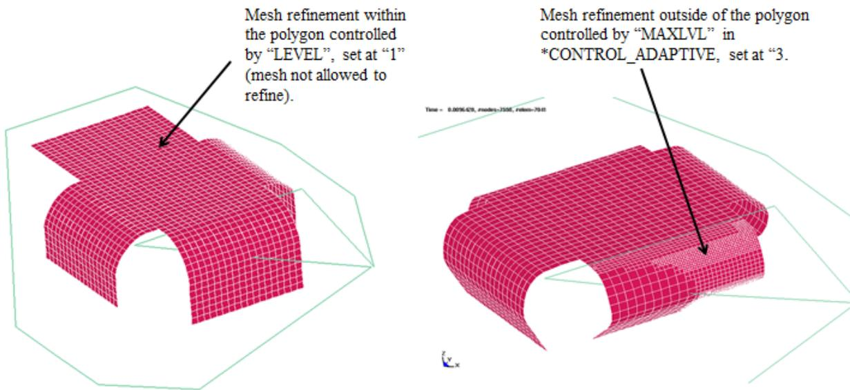
Figure 14. Mesh refinement when defined polygon curve exclude the area of interest, and LEVEL < MAXLVL.
