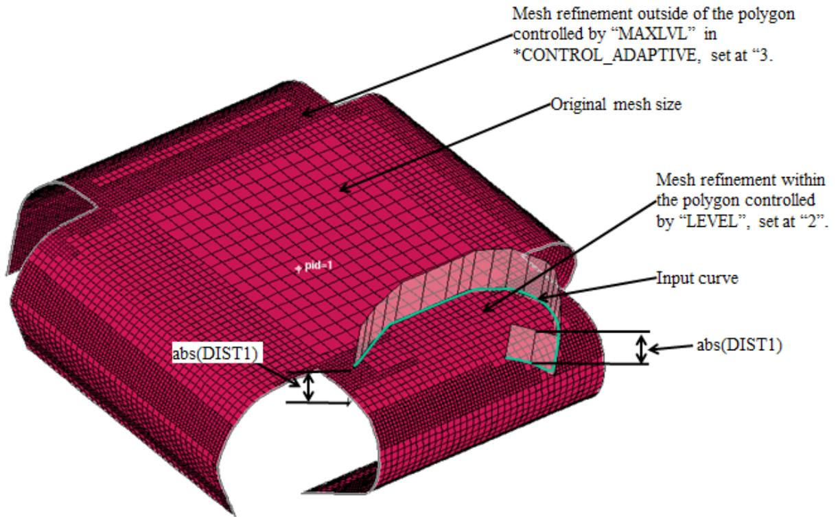
Figure 13. Mesh refinement when defined polygon curve enclose the area of interest, and MAXLVL≠1.
