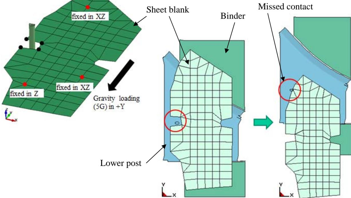
Figure 2. Missed contact between gaging pin and blank edge.
