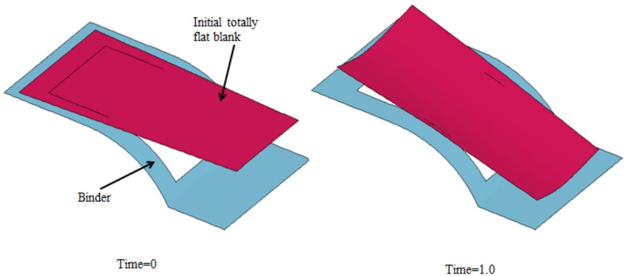
Figure 10. Switch from implicit dynamic to implicit static during gravity loading.
