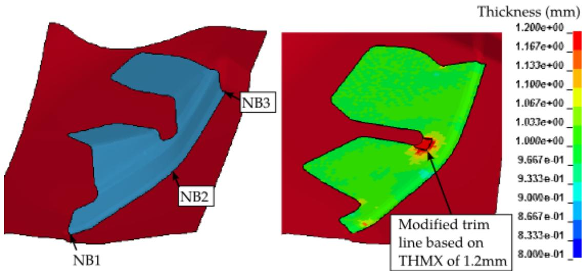
Figure 16. An example of flange before (left) and after (right) unfolding.
