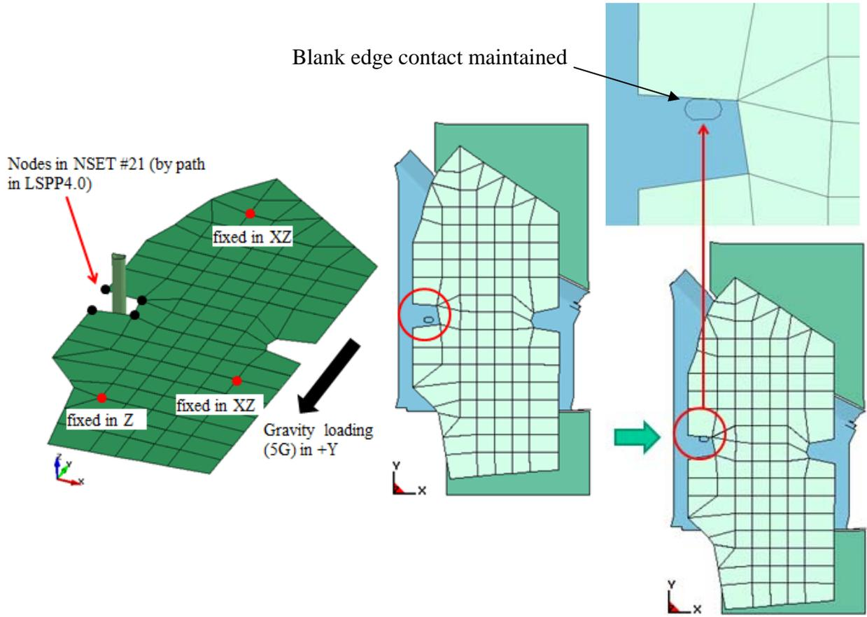
Figure 5. Blank edge/gage pin contact maintained with SOFT=6.
