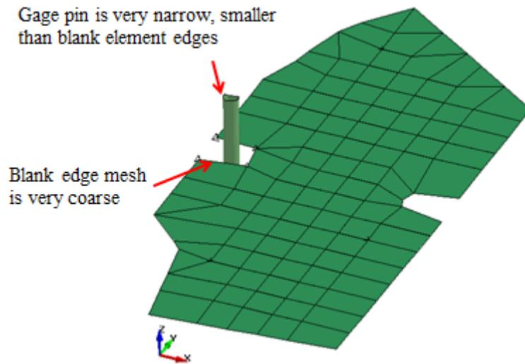
Figure 1. Gaging pin and blank mesh
