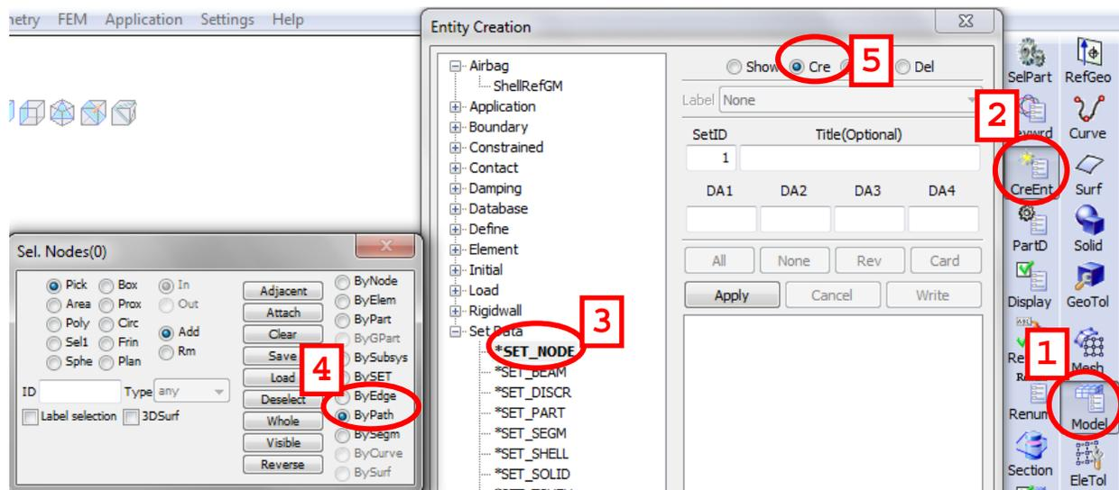
Figure 4. Create a node set "By Path" in LS-PrePost4.0.
