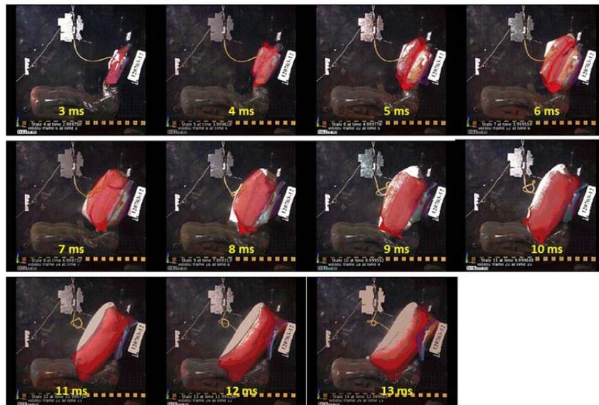
Figure 7. Static deployment shape of the single chamber SIAB. (a) deployment sequence using CV method, (b) deployment sequence using particle method, (c) comparison of sequence of particle method airbag deployment and test
