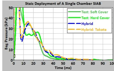
Figure 6. The static deployment airbag pressure profile using the airbag model delivered from a supplier and new airbag model after stripping off temperature scaling factor and other tuning factors.
