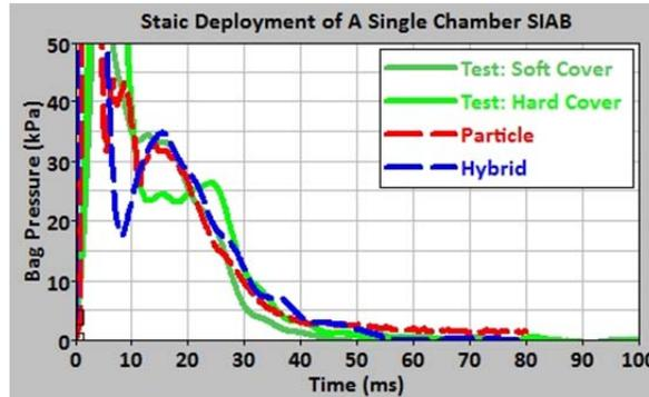
Figure A1. Static Deployment pressure history of using both particle and uniform pressure methods
