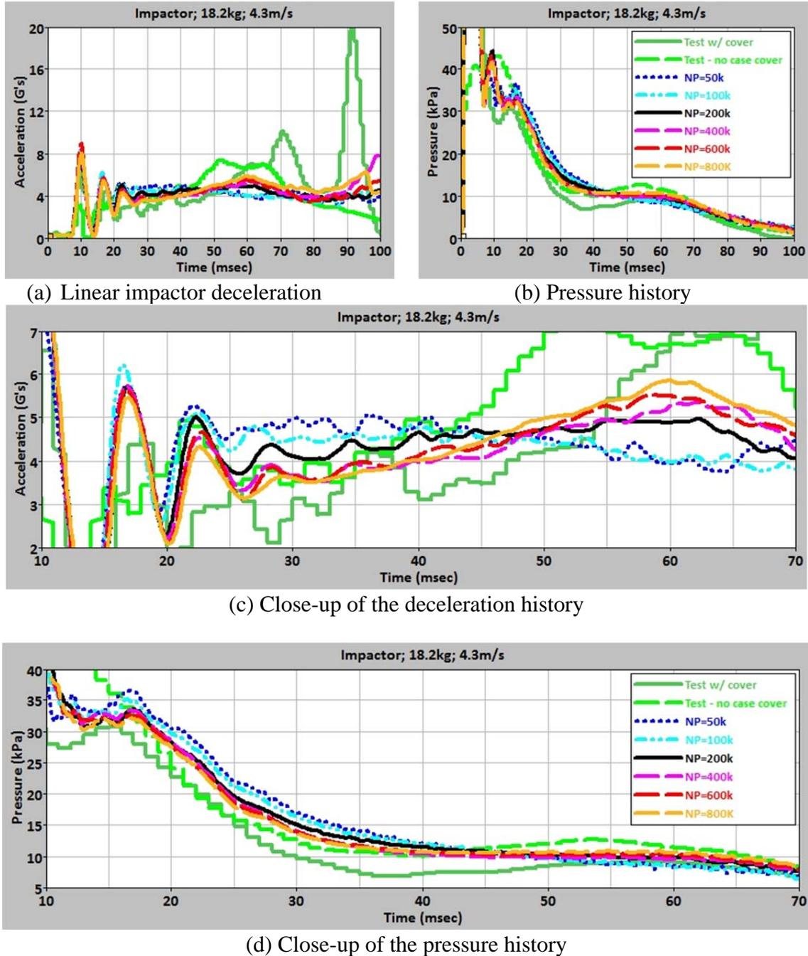
Figure 10. Impactor deceleration pulse and airbag pressure histories for 18.2kg impactor with 4.3m/s speed and 100mm distance from the airbag mounting plate to the reaction surface. (a) the deceleration history with NP (Number of Particles) ranging from 50k to 800k, (b) the associated pressure histories, (c) close-up of the deceleration history, (d) close-up of the pressure history.
