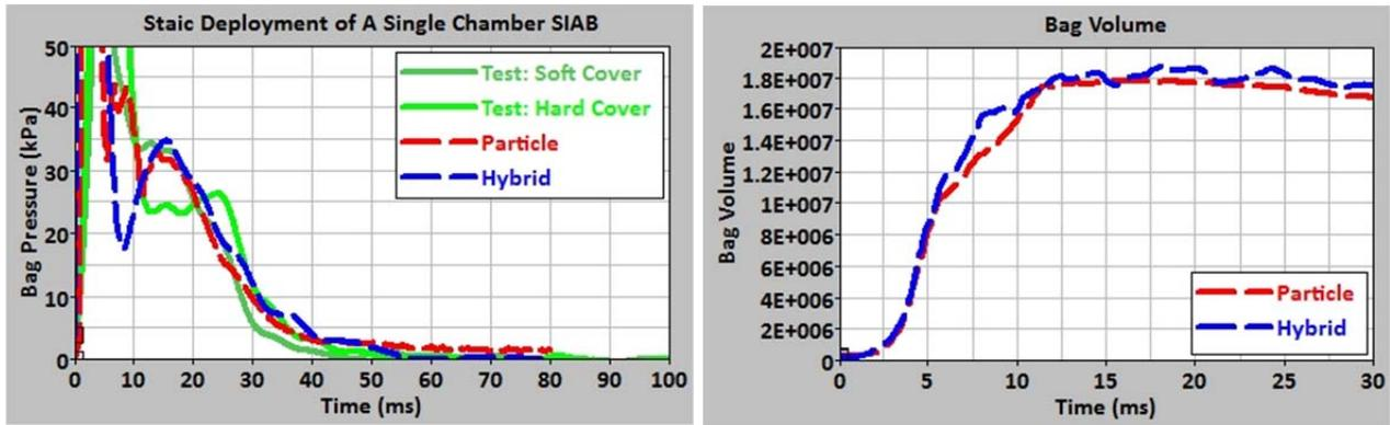
(a) airbag pressure test vs analysis
