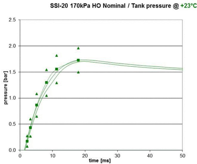
Figure 11. Pressure variation from the inflators' closed tank tests.
