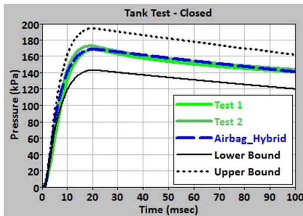
Figure 12. The upper and lower bounds of the pressure curves were replicated by adjusting the inflator temperature curve in the model by +/-14%.
