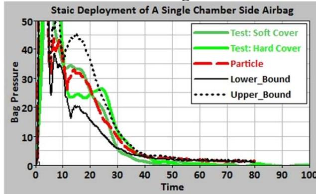
Figure B1. Static Deployment pressure history of using both particle and uniform pressure methods
