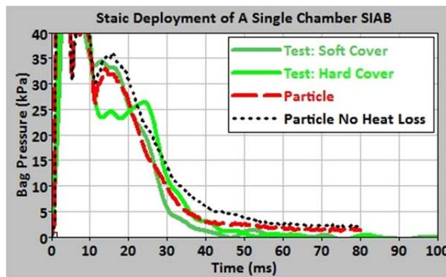
Figure 5. Static deployment of side impact airbag using particle method with and without considering the heat loss through fabric.
