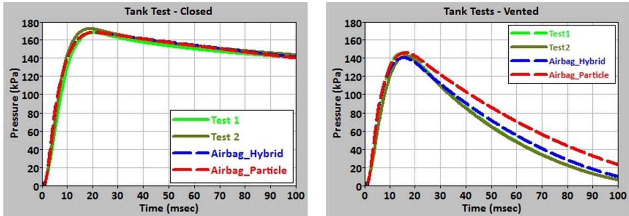
(a) Closed tank test
