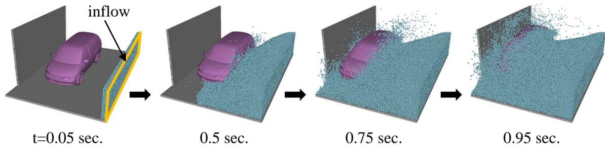
Fig.12 Result of tsunami simulation using MPS
