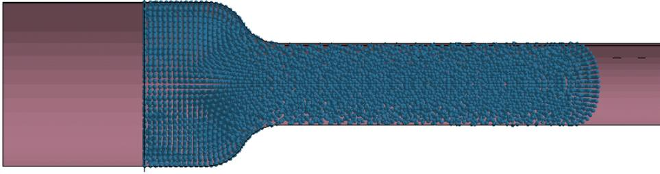
Fig.5 "push-in" analysis to simulate Newtonian viscous flow in SPH
