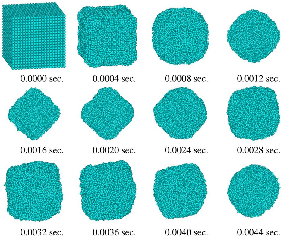
Fig.7 Shape change caused by CSF model of 1mm × 1mm × 1mm water cube
