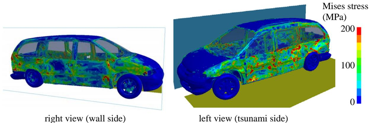
Fig.14 Deformation and Mises stress distribution of the vehicle at 1.0 second.
