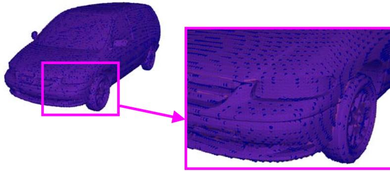
Fig.11 STL vehicle geometry and generated rigid particle of vehicle for MPS simulation
