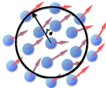
Fig.1 MPS kernel function
