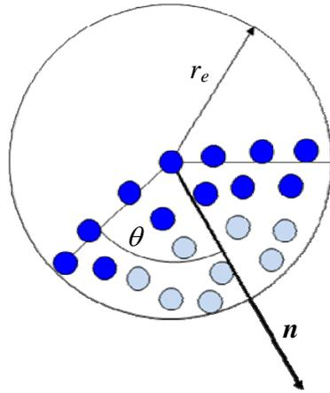
Fig.6 Surface tension model in MPS
