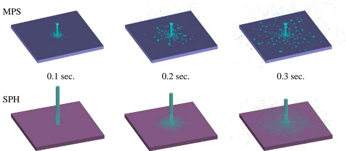
Fig.8 Water splay on flat plate
