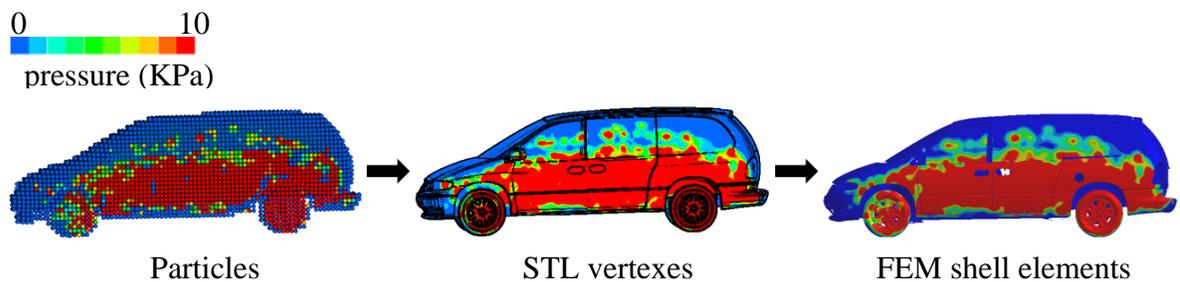
Fig.13 Example of mapping result of pressure distribution at time = 0.85 sec.
