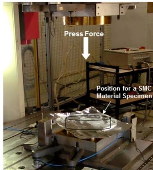
Figure 1 Long fiber SMC press rheometry testing experimental set-up at IVW GmbH
