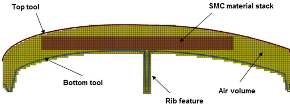
Figure 8 Two dimensional SMC compression spoiler tool model developed in LS-DYNA
