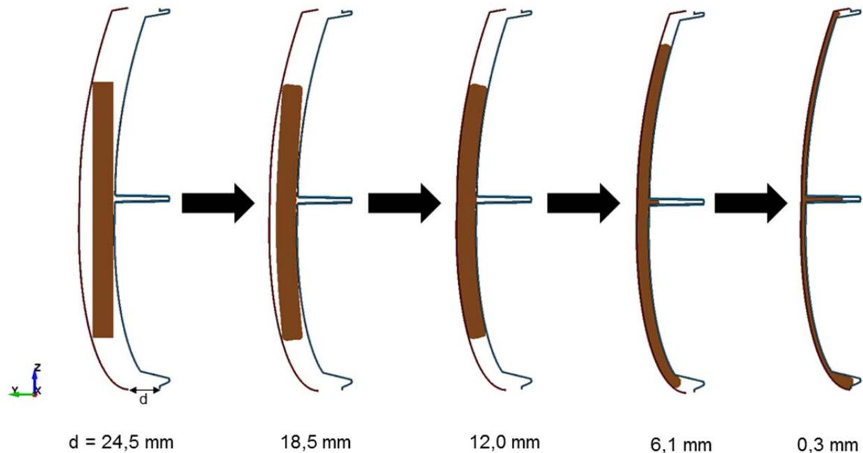
Figure 9 Animation states showing the various stages of SMC compression and flow in the two-dimensional automotive spoiler model.
