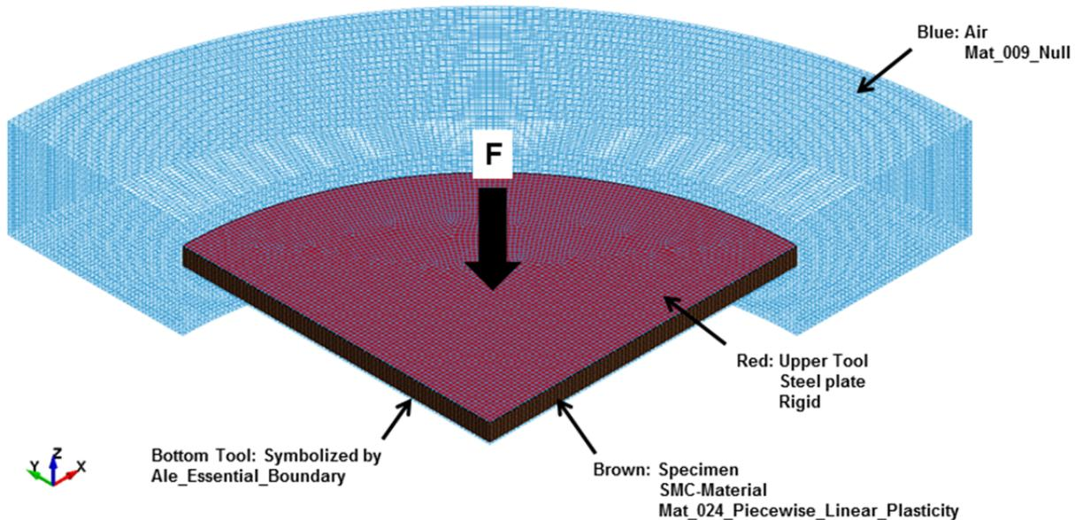
Figure 3 ALE-Formulation of the press rheometry characterization test setup in LS-DYNA
