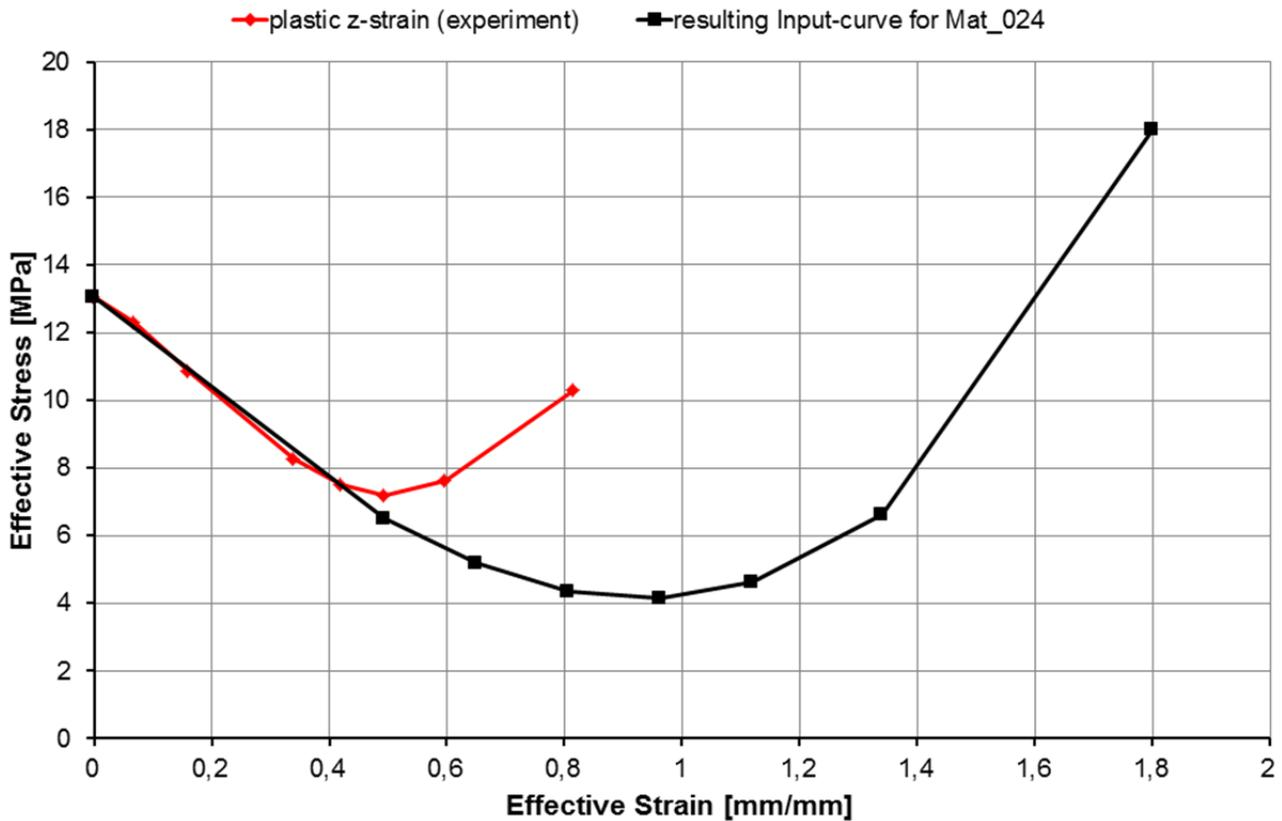
Figure 4 Resulting input curve for Mat\_024 plastic stress- strain compared to the experimental data
