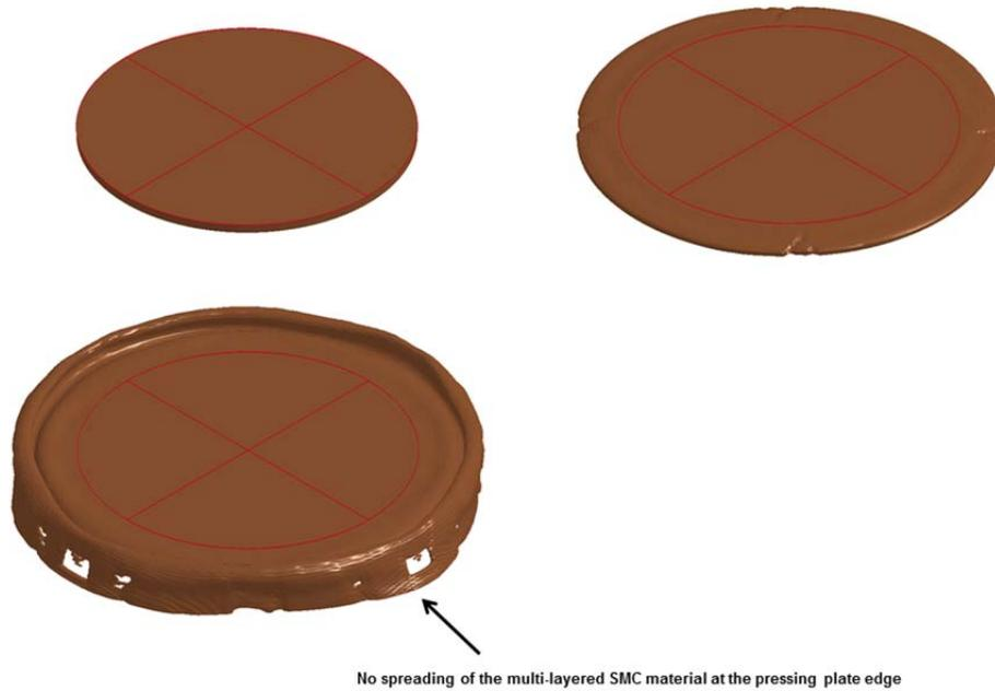
Figure 6 Simulated and actual press rheometry SMC material combined compression and flow deformation
