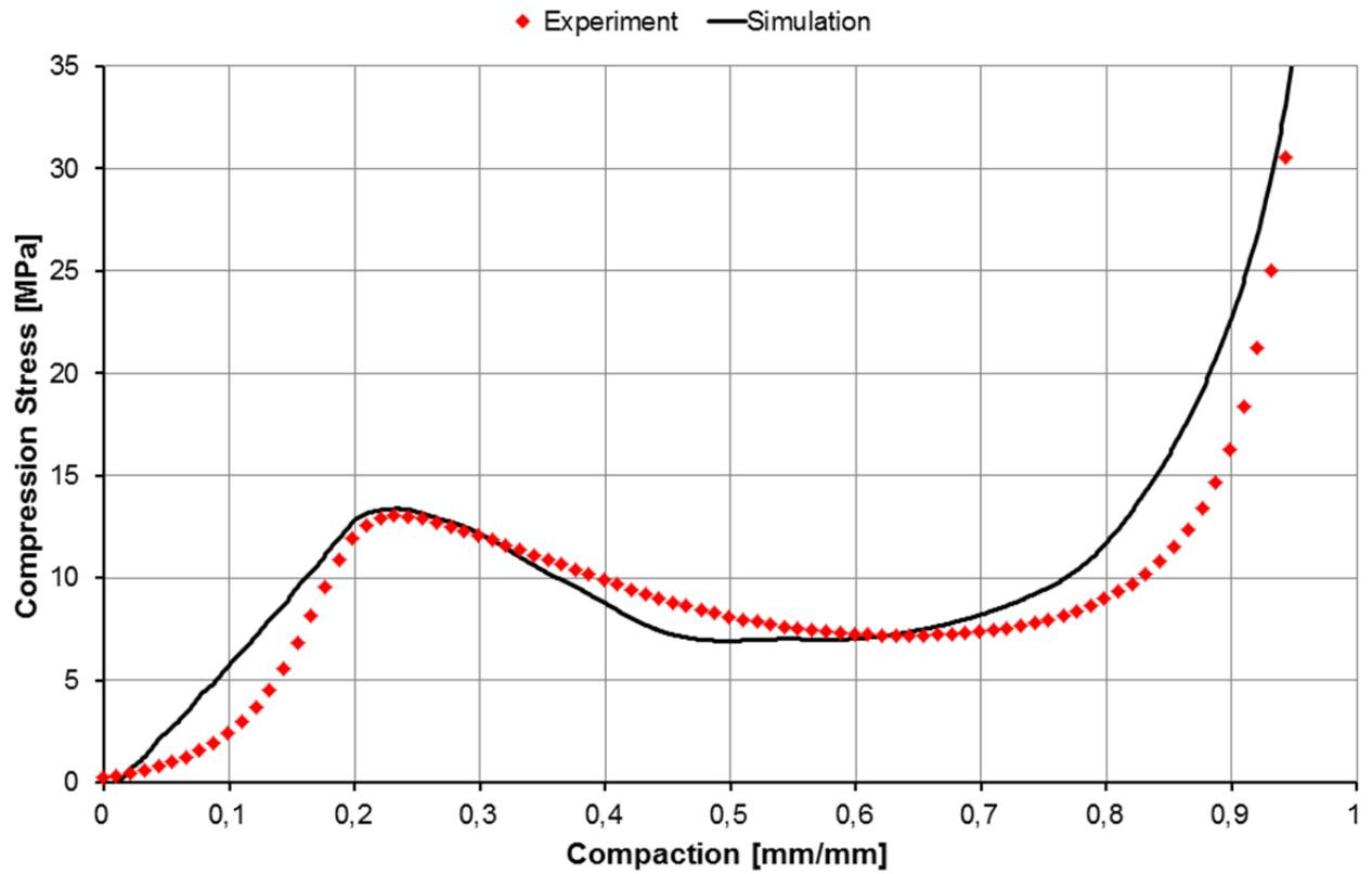
Figure 5 Comparison of experimental and simulated compression stress versus compaction curves
