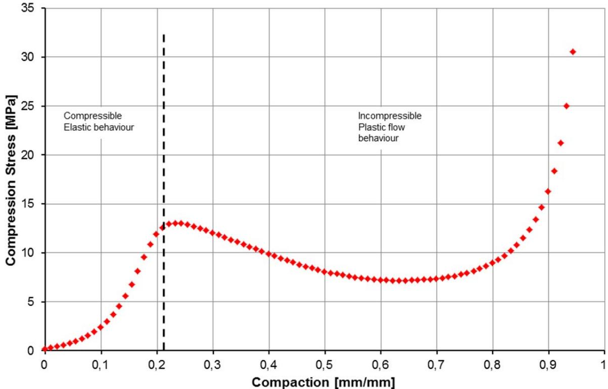
Figure 2 Typical compression stress versus compaction for measured SMC material
