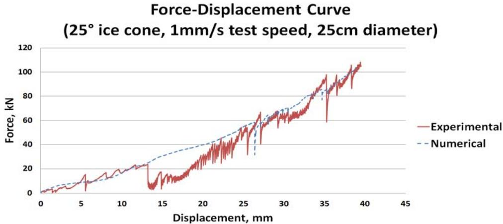
Figure 11: Comparison of force-displacement curve (25cm ice cone, 1mm/s test speed)
