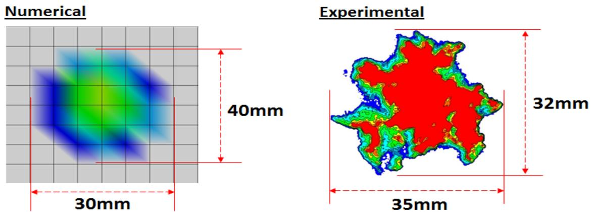
(a) Spatial pressure distribution at test step 1 (at displacement=9mm)
