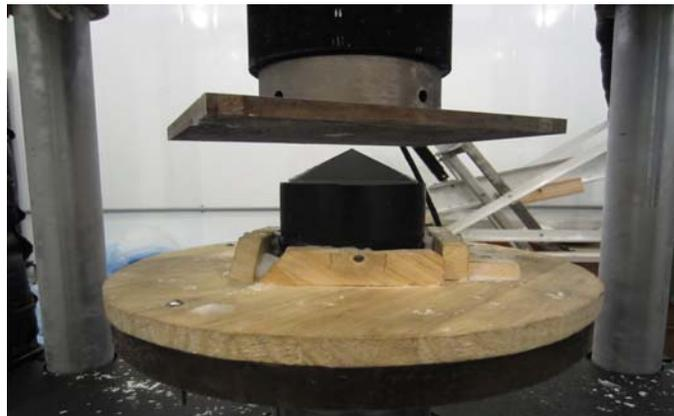
Figure 6: Test set-up (left: 30° ice cone, right: 50° ice cone)
