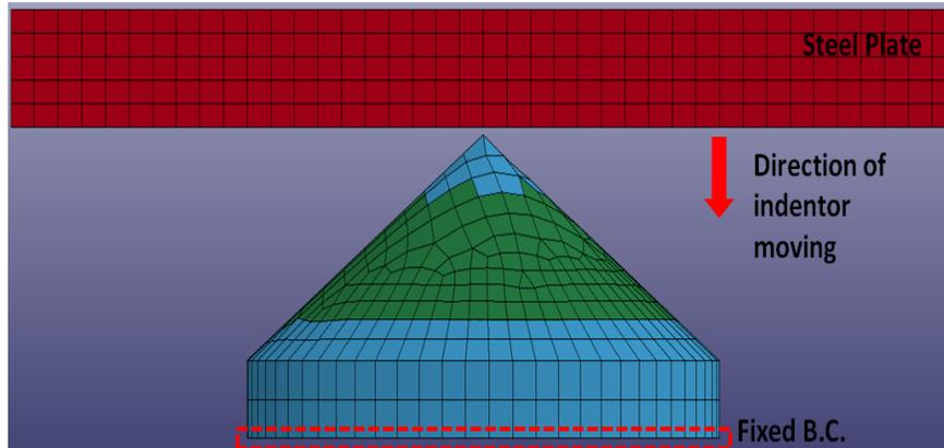
Figure 5: Numerical simulation model consist of ice specimen and steel plate
