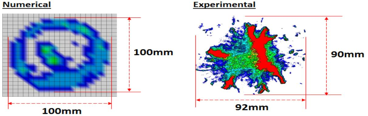
(c) Spatial pressure distribution at test step 3 (at displacement=27mm)
