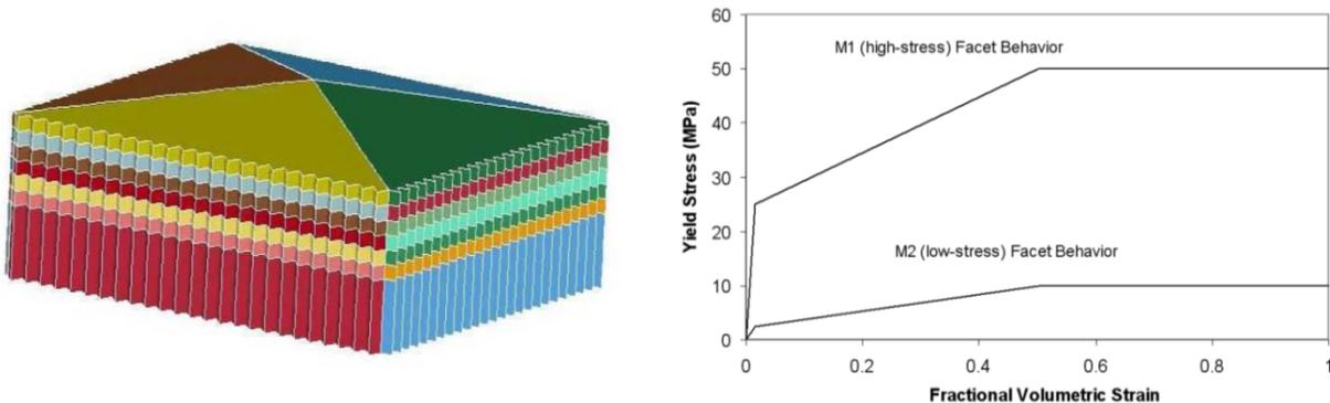
Figure 2: View of the numerical model (left), volumetric strain stress curves for crushable foam (right) [5] [6]
