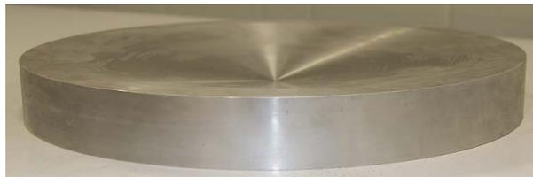
Figure 10: 10° conical shape indenter
