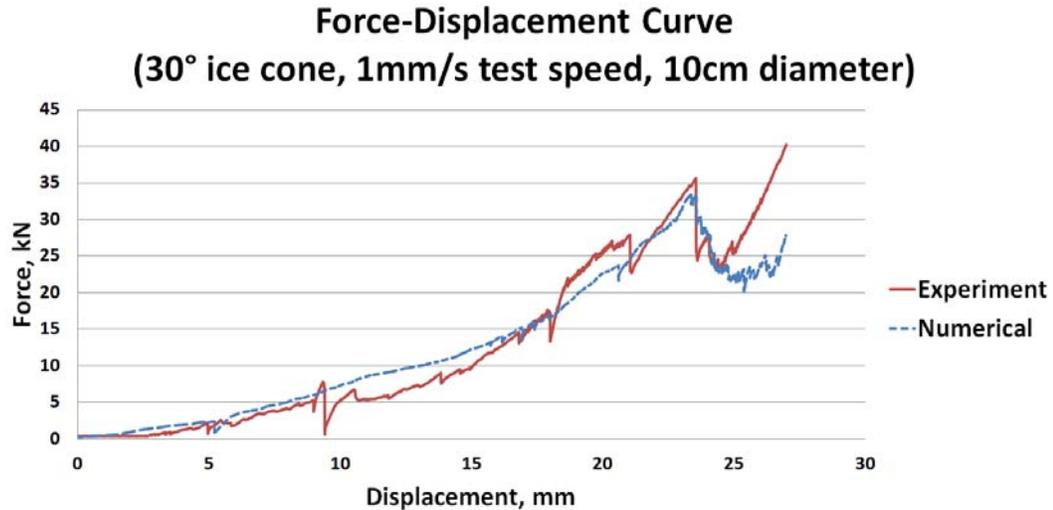
Figure 7: Comparison of force-displacement curve (1mm/s test speed)
