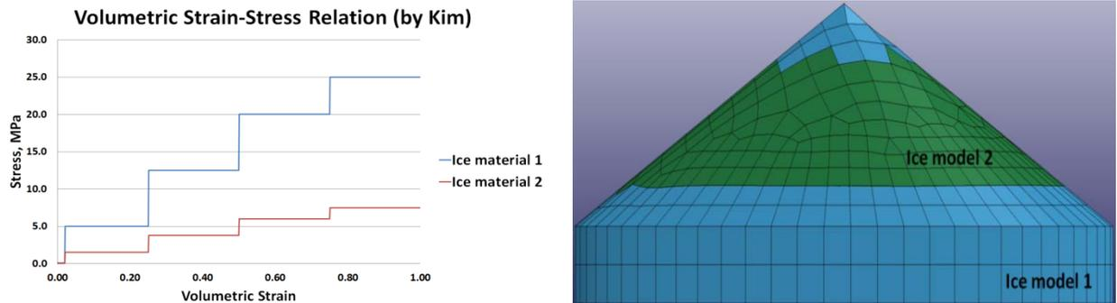
Figure 4: Volumetric strain-stress relation of crushable foam (left), layer of ice model (right)
