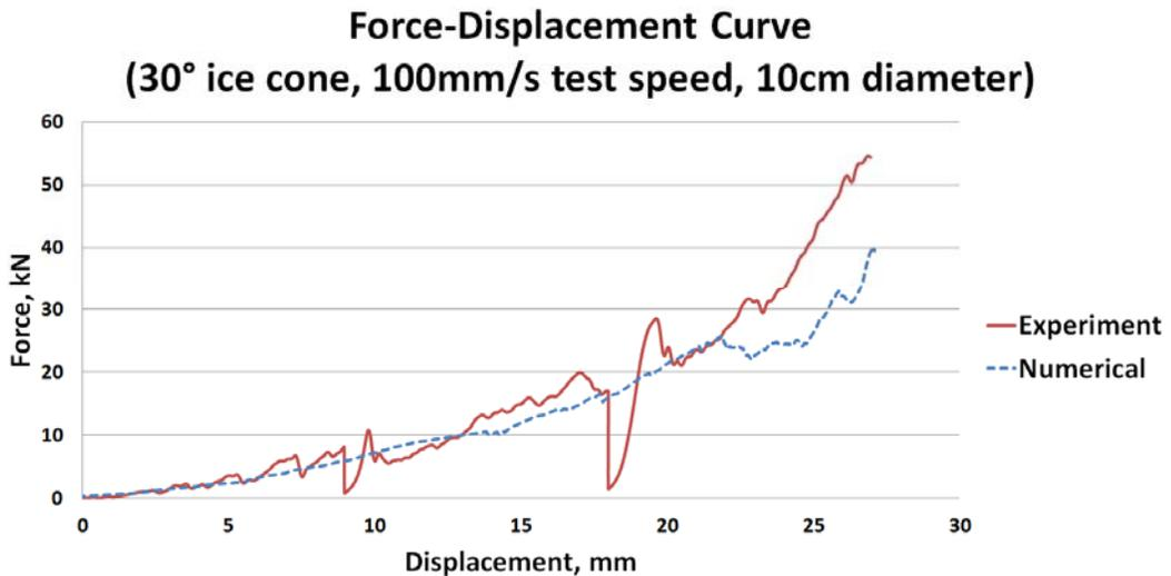
Figure 8: Comparison of force-displacement curve (100mm/s test speed)
