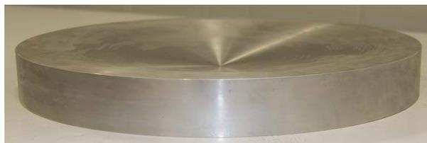
Figure 10: 10° conical shape indenter
