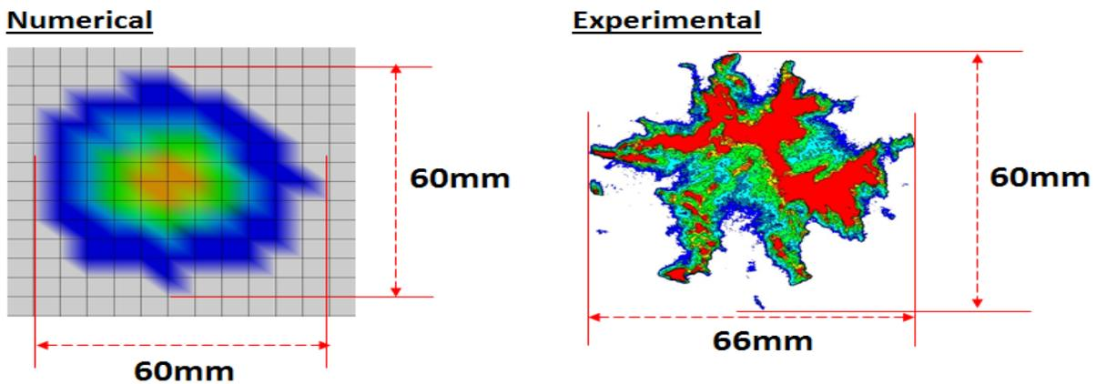
(b) Spatial pressure distribution at test step 2 (at displacement=18mm)
