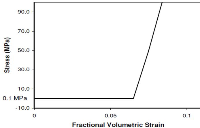
Figure 1: Volumetric strain-stress relationship [3]
