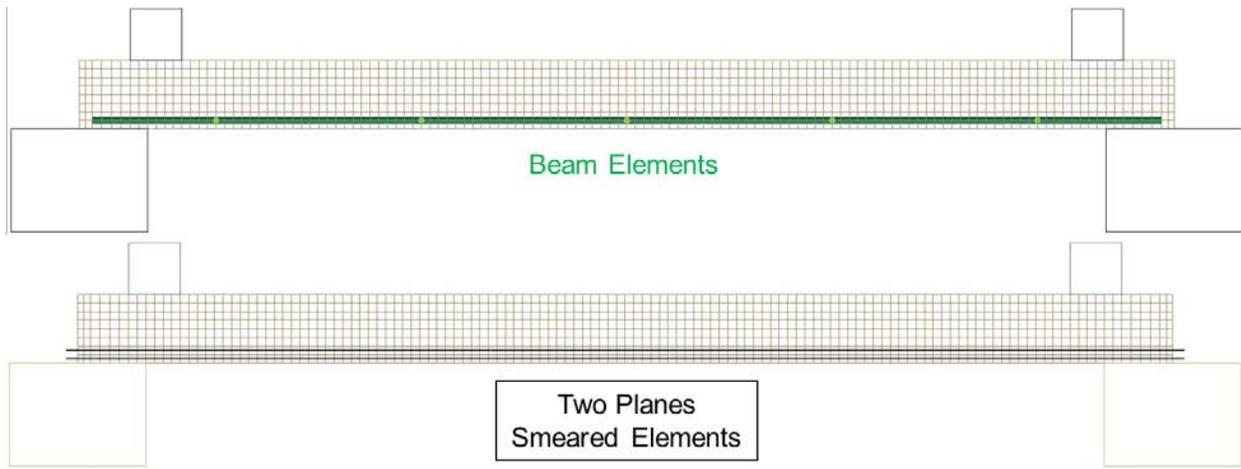
Figure 5 Illustration of two (bottom) rows of concrete elements occupied by the explicit beam element reinforcement or the smeared reinforcement.
