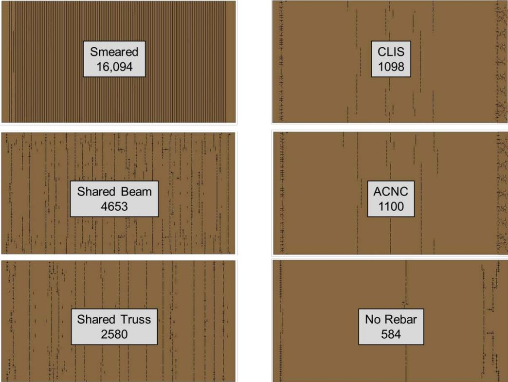
Figure 10 Illustration of crack patterns and number of cracks for the various methods of including rebar in a slab under axial extension.
