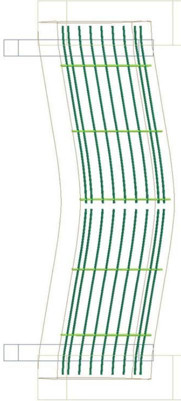
Figure 21 Failure of reinforcement after about 20ms.
