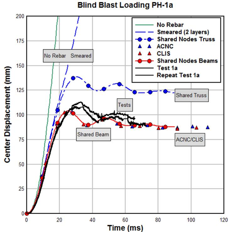
Figure 13 Slab central displacement under blast loading for five different rebar methods compared to the two repeat experimental results.
