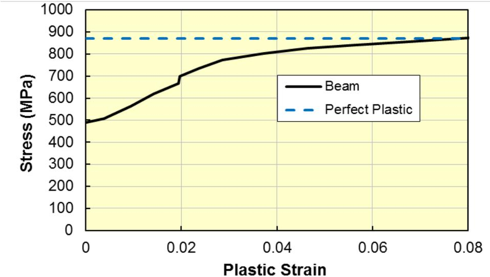
Figure 7 Elastic-perfect plastic assumed constitutive model for reinforcement/
