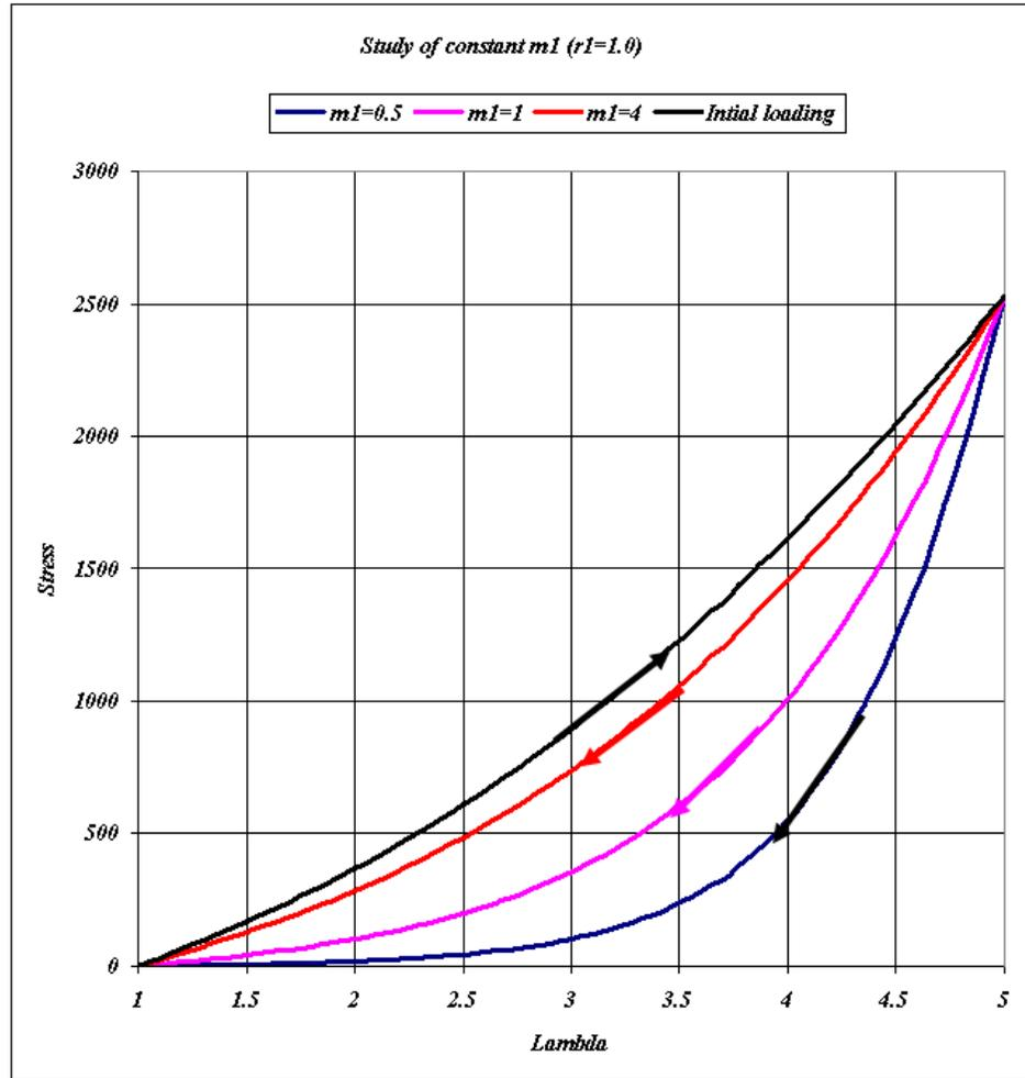
Figure 3. The effect of  $m_1$  on unloading for uniaxial extension
