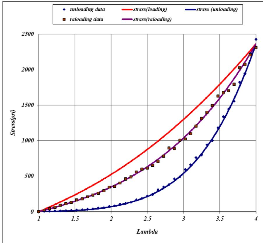
Figure 5. The best-fit unloading and reloading stress-stretch curves and the test data
