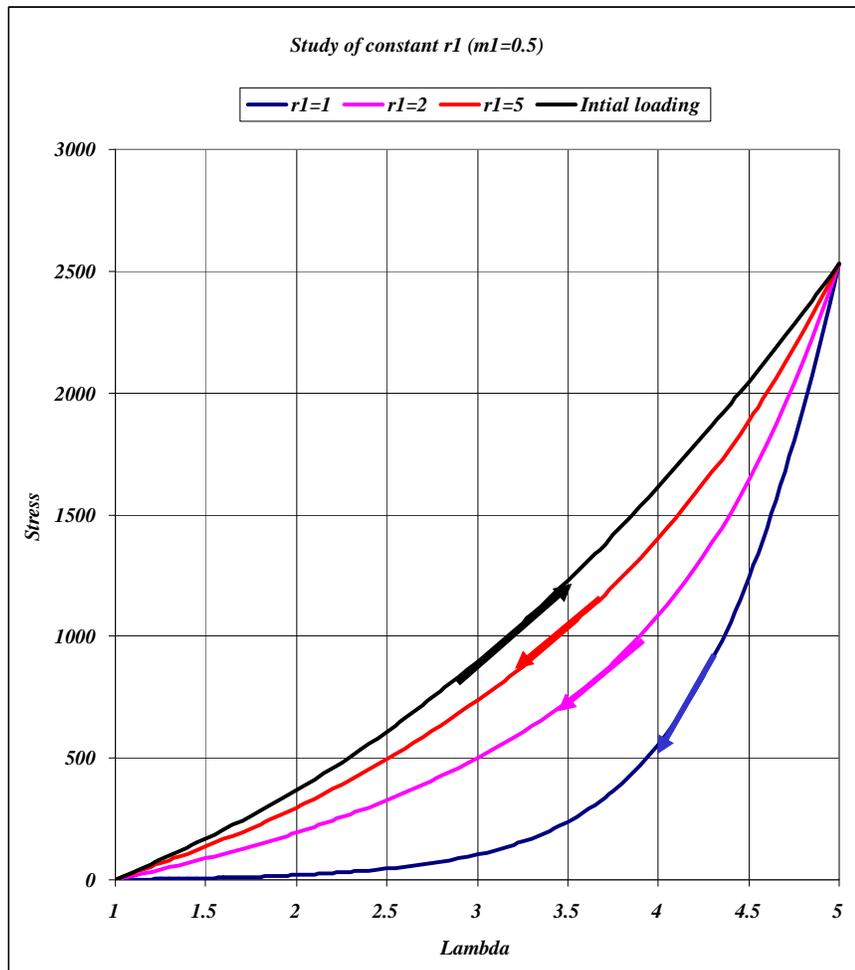
Figure 2. The effect of  $r_1$  on unloading for uniaxial extension
