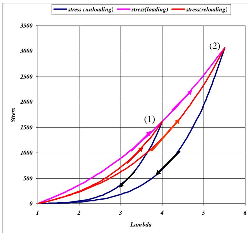
Figure 1. The Mullins effect for uniaxial loading, unloading and subsequent reloading, obtained from EXCEL.
