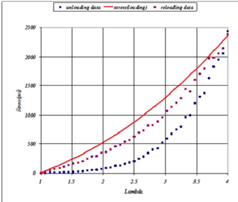
Figure 4. The stress-stretch curve for a neo-Hookean material and the numerical generated test data for unloading and reloading.
