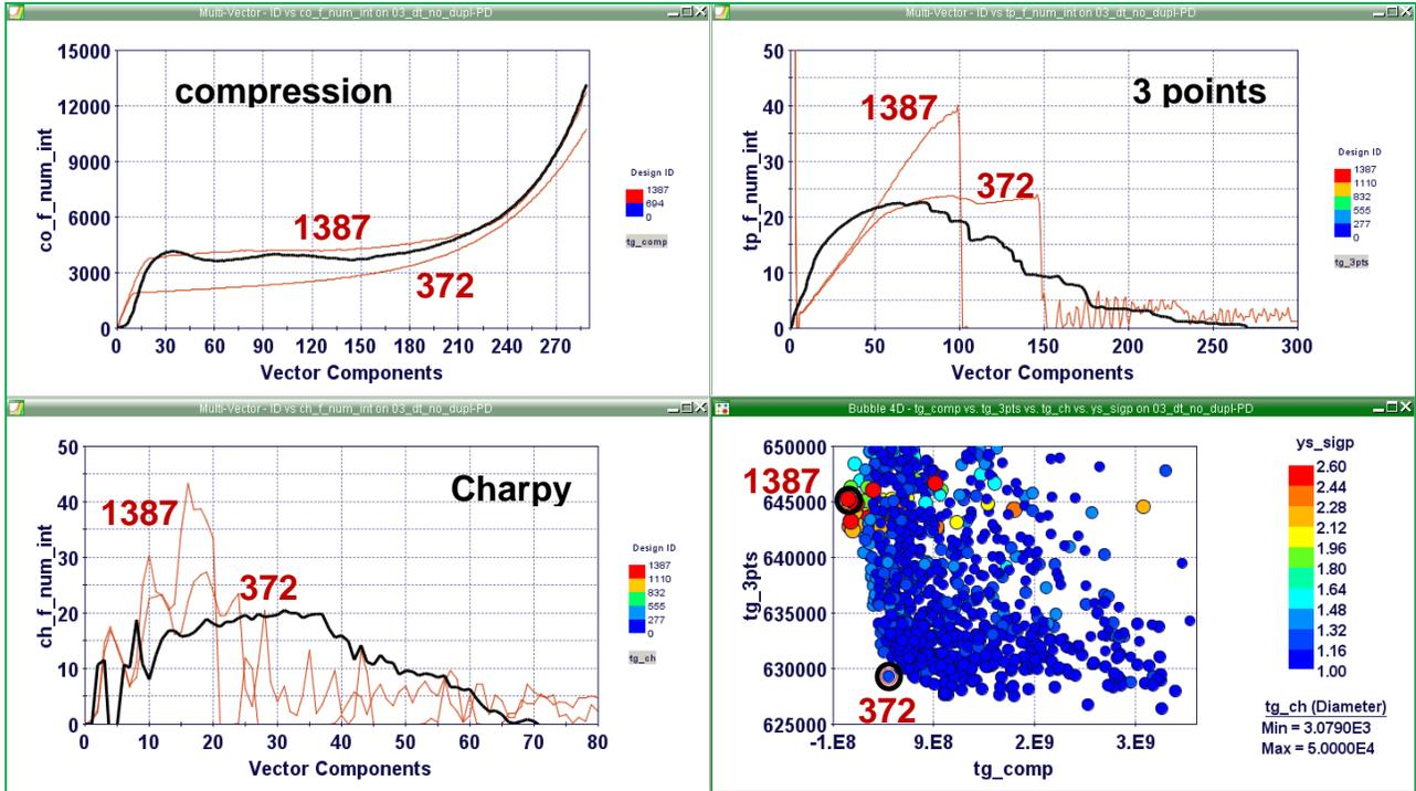
Figure 23: two trade-off solutions between all three FE models – des 372 and 1387
