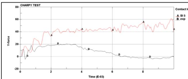
Figure 18: des 7148 – Charpy pendulum with Cal\_Mod CFAIL=0 (no failure)
