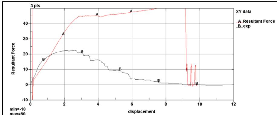
Figure 3: 3 pts bending with Cal\_Mod
