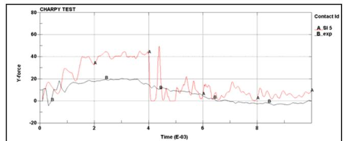
Figure 19: des 7148 – Charpy pendulum with Cal\_Mod CFAIL=0.2
