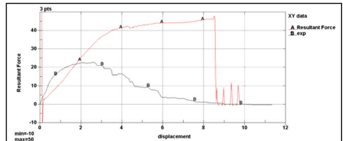
Figure 17: des 7148 – 3 pts bending with Cal\_Mod CFAIL=0.2
