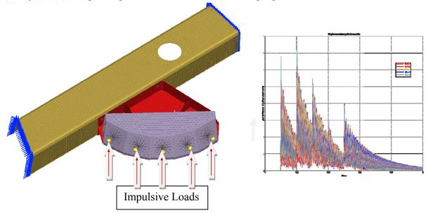
Resultant displacement is plotted. Time for explicit transient analysis is 3.5 hours. Using Modal Dynamics the run time is reduced to 3.5 minutes. Most of the savings is due to an almost 1000 times increase in the time step reducing the number of time steps by 1000.
