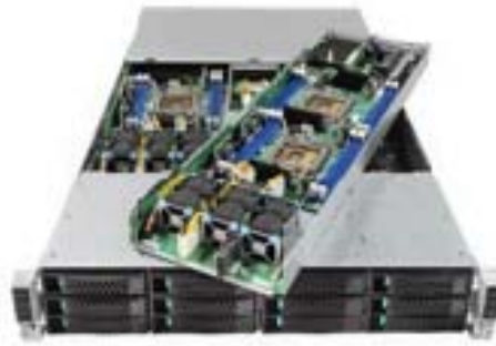
Figure 1: Overhead View of SGI Rackable Server with the Top Cover Removed
